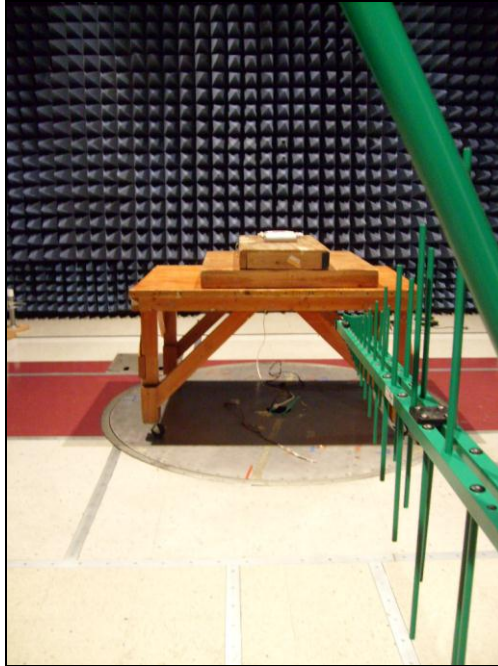
Photograph 2. Radiated Emission Spurious Test Setup, 30 MHz – 1 GHz
