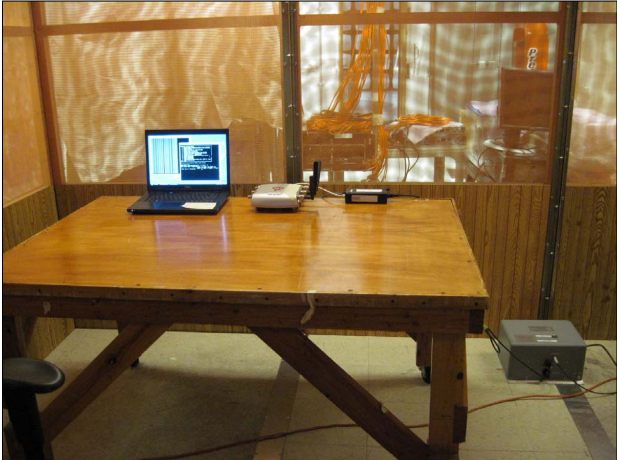
Photograph 3. Conducted Emissions, Test Setup PoE30U-560
