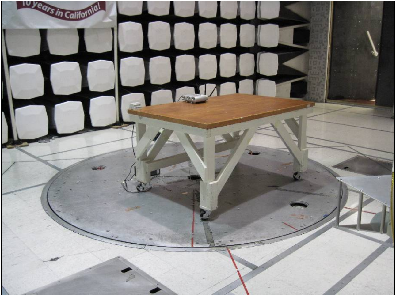
Photograph 4. Radiated Emission, Test Setup
