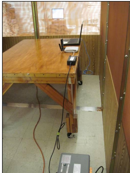
Photograph 6. Conducted Emissions, Test Setup 2, PoE30U-560
