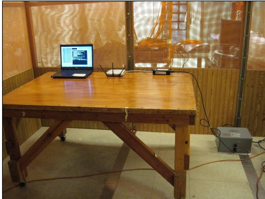
Photograph 5. Conducted Emissions, Test Setup 1, PoE30U-560
