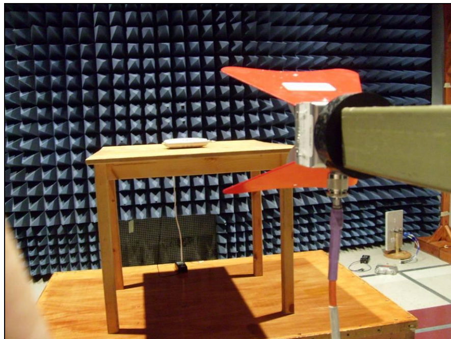
Photograph 3 Radiated Emission Spurious Test Setup, 1 GHz – 18 GHz
