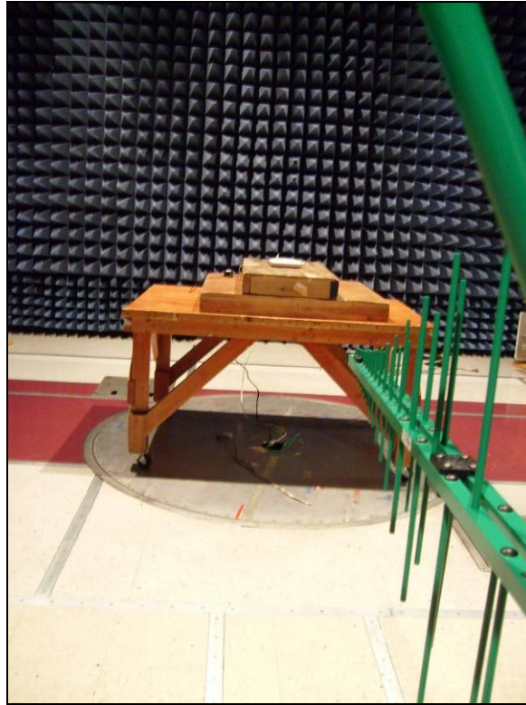
Photograph 2. Radiated Emission Spurious Test Setup, 30 MHz – 1 GHz
