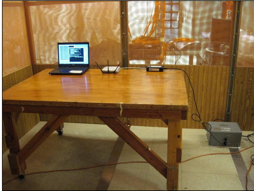
Photograph 4. Conducted Emissions, PoE30U-560, Test Setup 1
