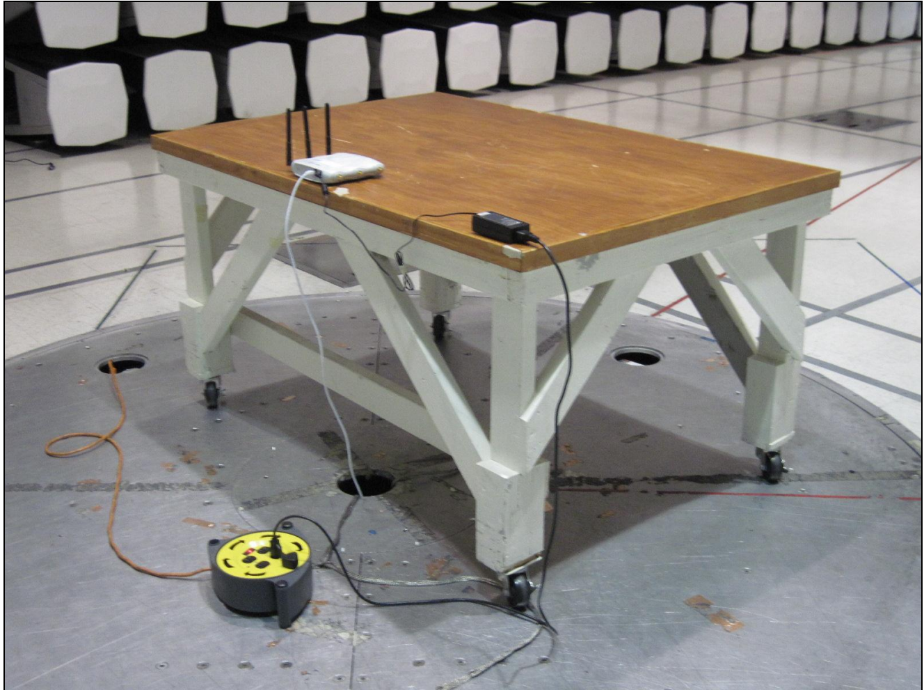
Photograph 6. Radiated Emission, Test Setup
