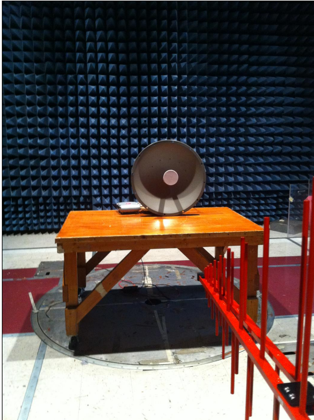
Photograph 1. Radiated Spurious Emissions, Test Setup, 30 MHz – 1 GHz
