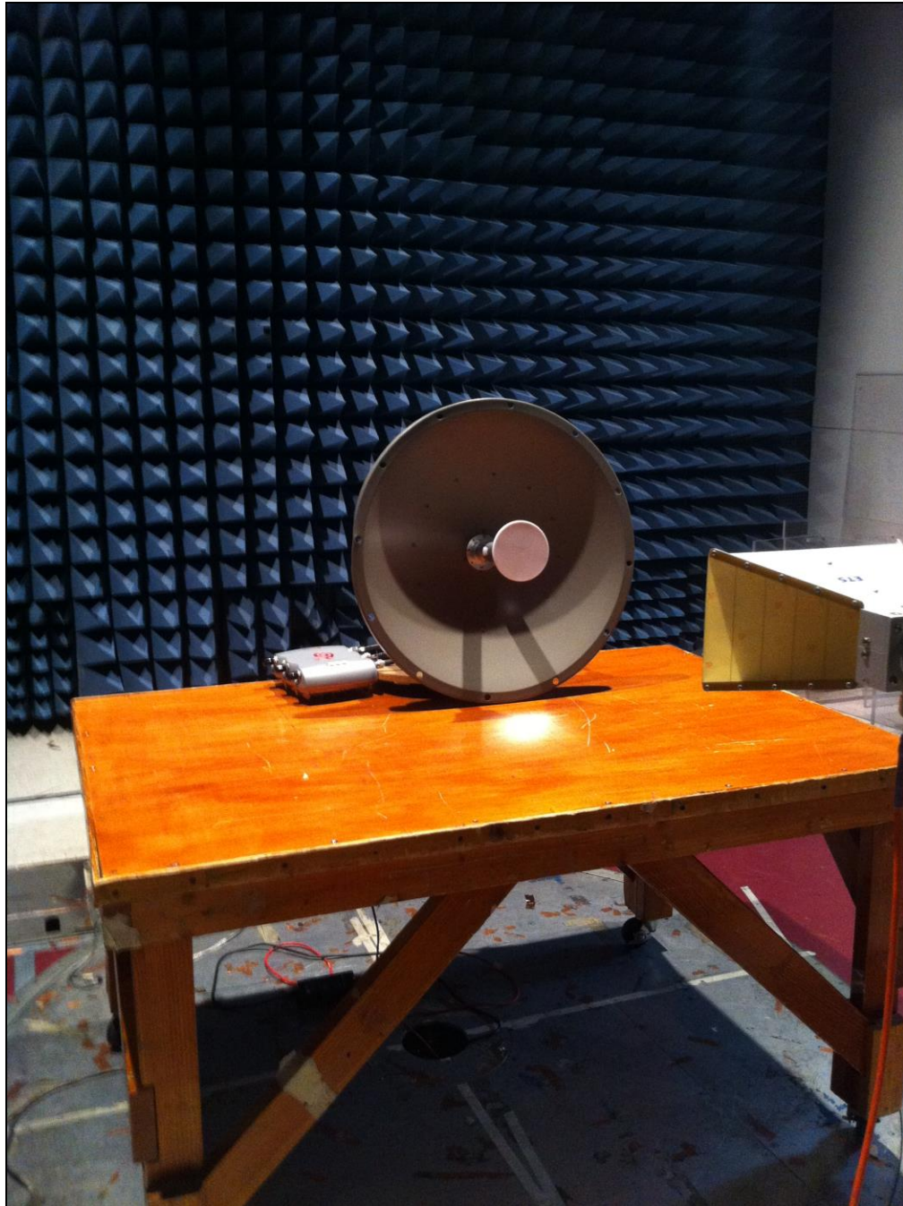
Photograph 2. Radiated Spurious Emissions, Test Setup, 1 GHz – 18 GHz
