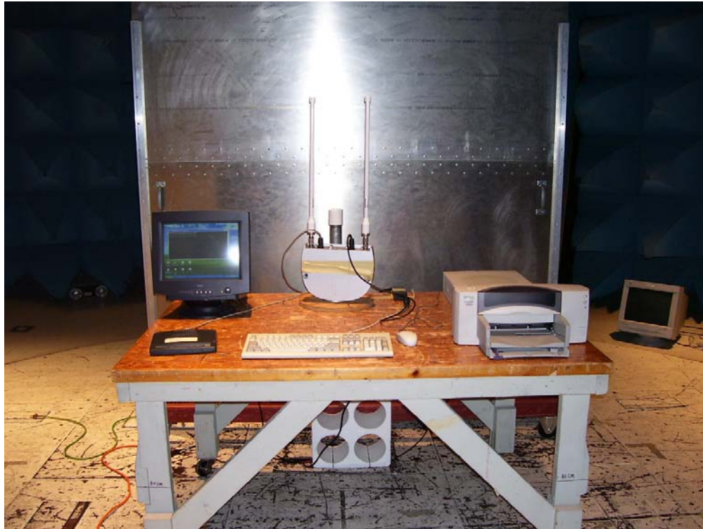
Photograph 5. Conducted Emissions Test Setup
