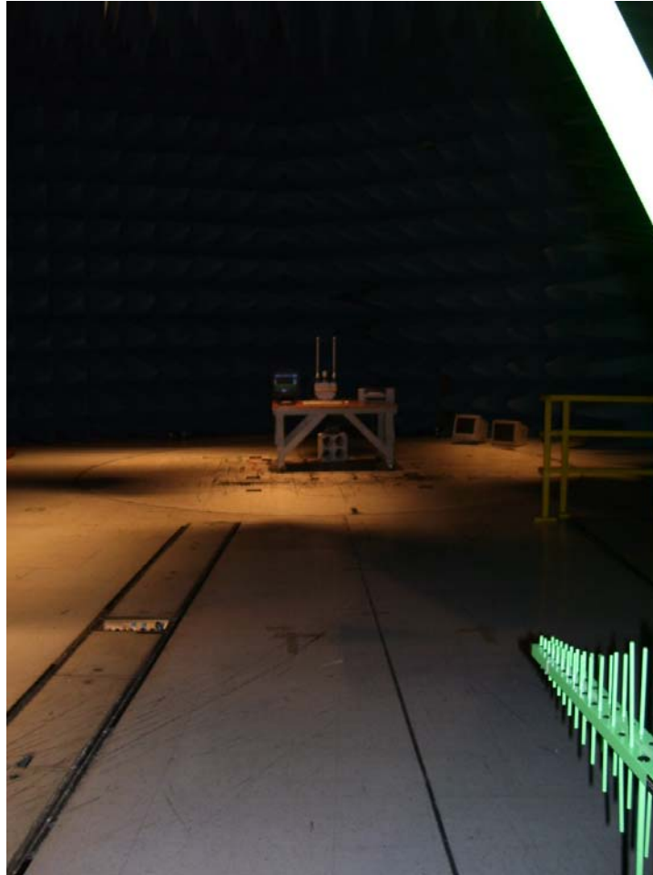
Photograph 3. Radiated Emission Test Setup 30 MHz - 1 GHz
