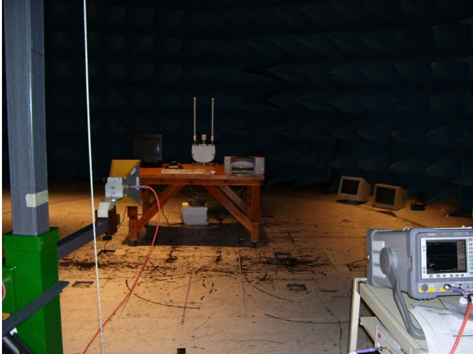
Photograph 4. Radiated Emission Limits Test Setup 1 - 2GHz
