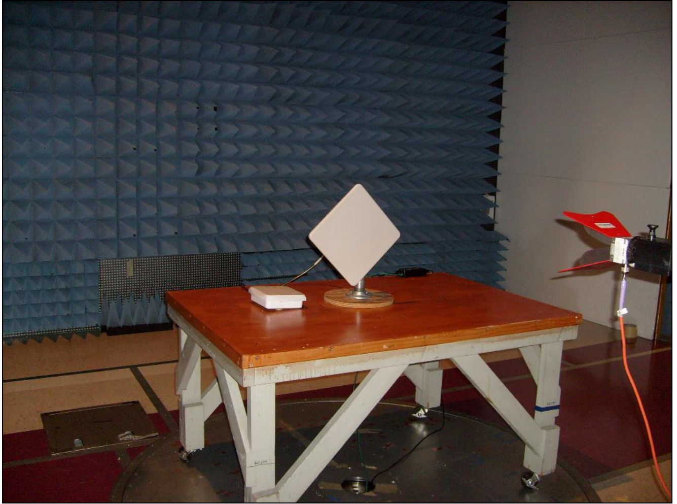
Photograph 7. Radiated Emissions, 1 GHz – 18 GHz @ 1m, 23 dBi Panel
