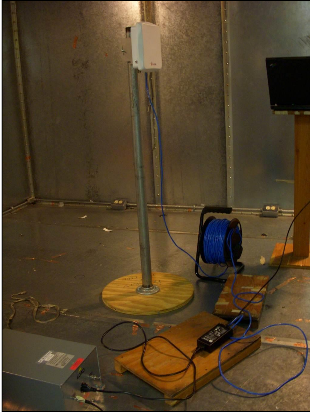
Photograph 3. Conducted Emissions, Test Setup
