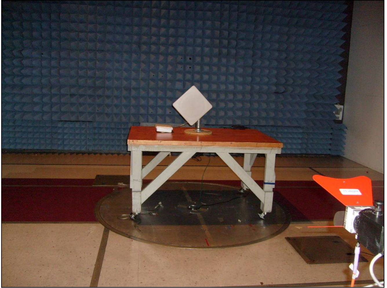
Photograph 11. Radiated Emissions, 1 GHz – 18 GHz @ 3m, 23 dBi Panel
