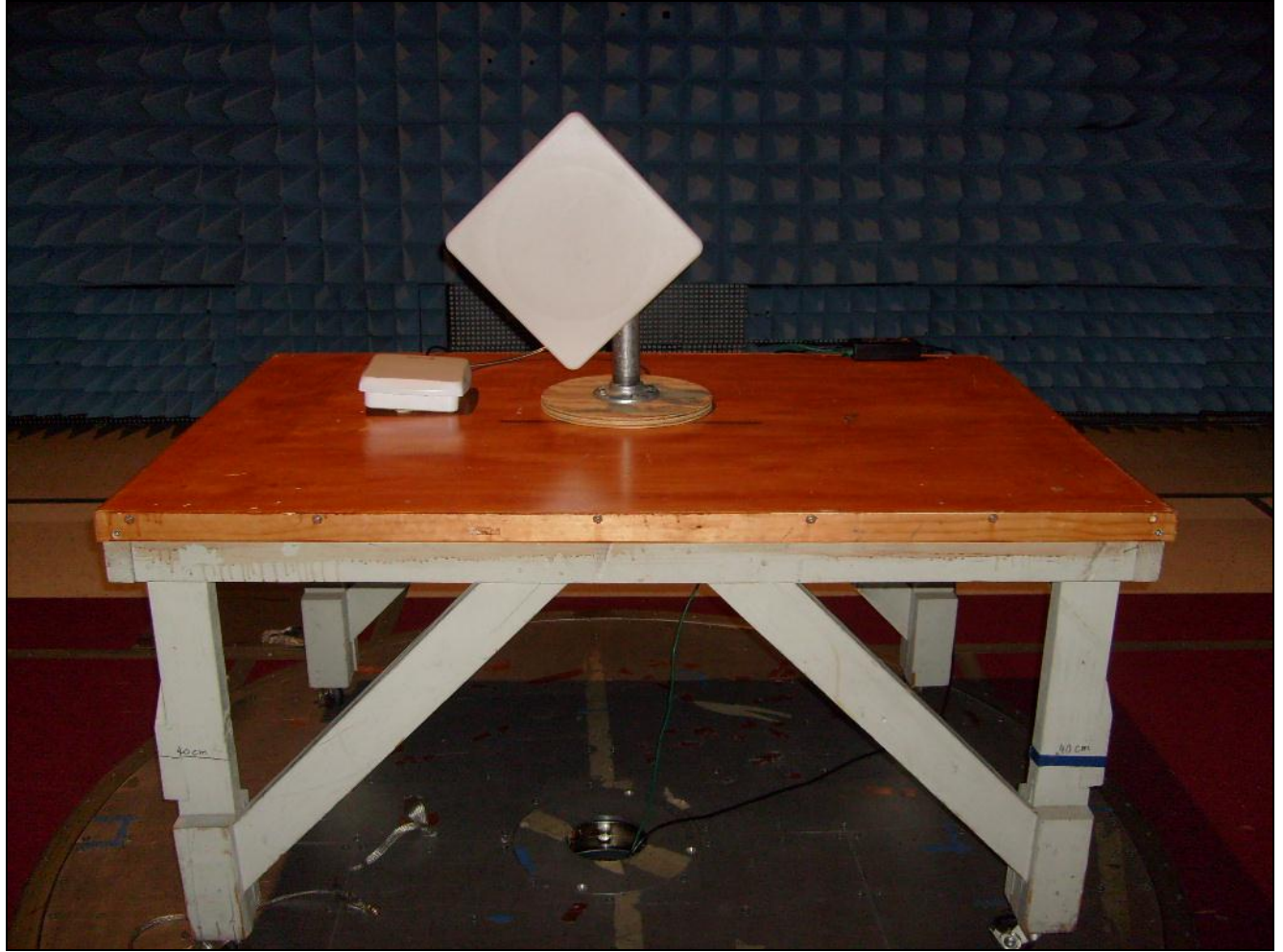
Photograph 8. Radiated Emissions, 23 dBi Panel, Test Setup
