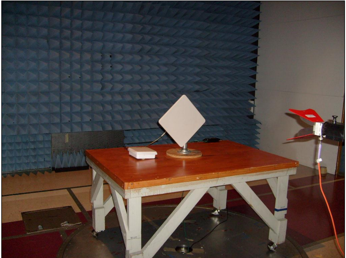
Photograph 5. Radiated Emissions, 1 GHz – 18 GHz @ 1m, 23 dBi Panel
