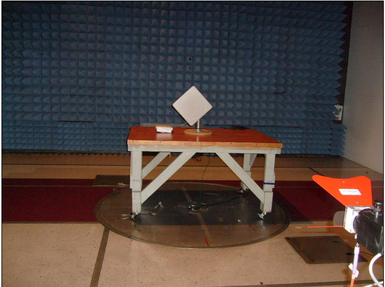
Photograph 9. Radiated Emissions, 1 GHz – 18 GHz @ 3m, 23 dBi Panel
