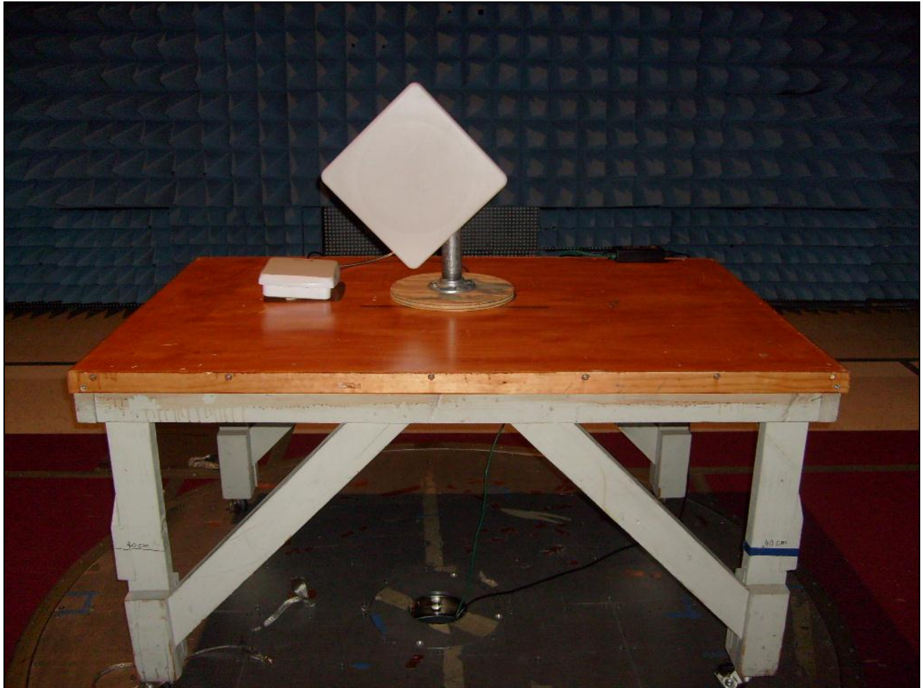
Photograph 6. Radiated Emissions, 23 dBi Panel, Test Setup
