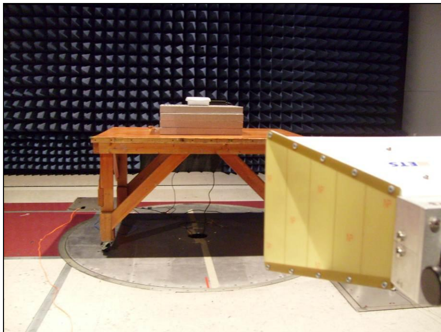
Photograph 3 Radiated Emission Spurious Test Setup, 1 GHz – 18 GHz
