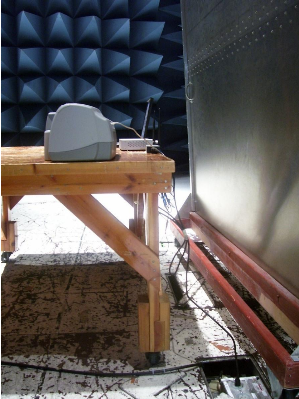
Photograph 1. Conducted Emissions, Test Setup
