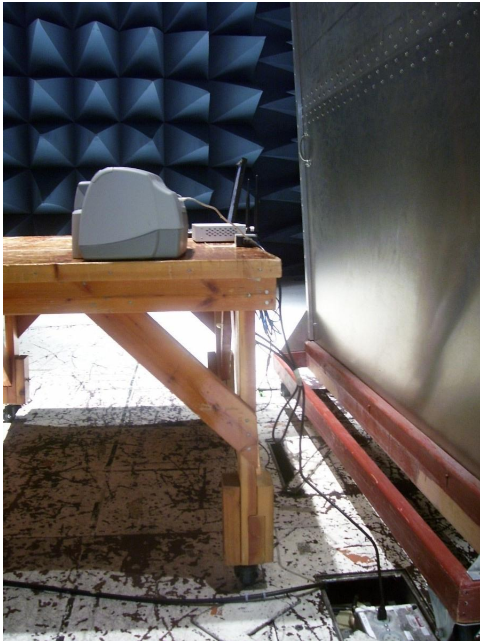
Photograph 1. Conducted Emissions, Test Setup
