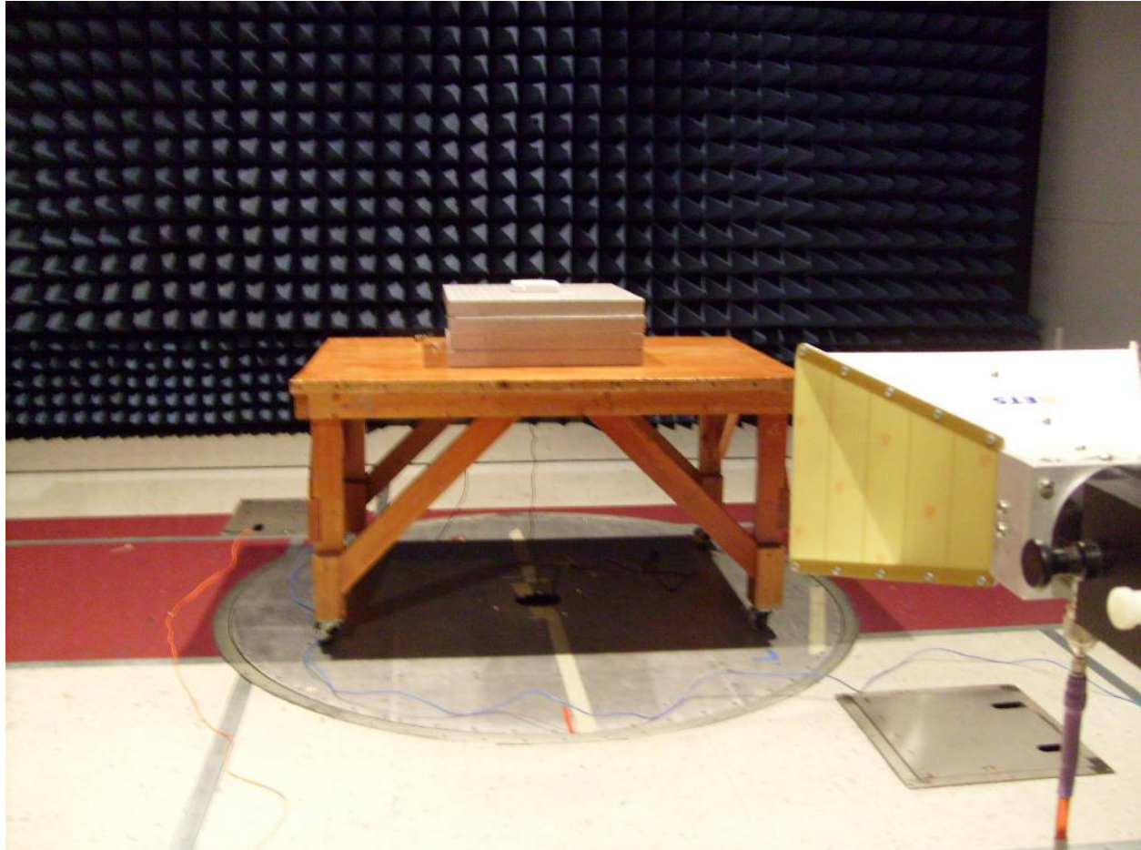
Photograph 3. Radiated Measurements Test Setup (1GHz-18GHz)
