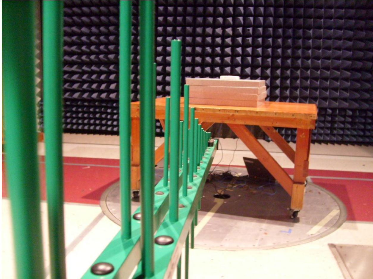
Photograph 2. Radiated Measurements Test Setup (30MHz-1GHz)
