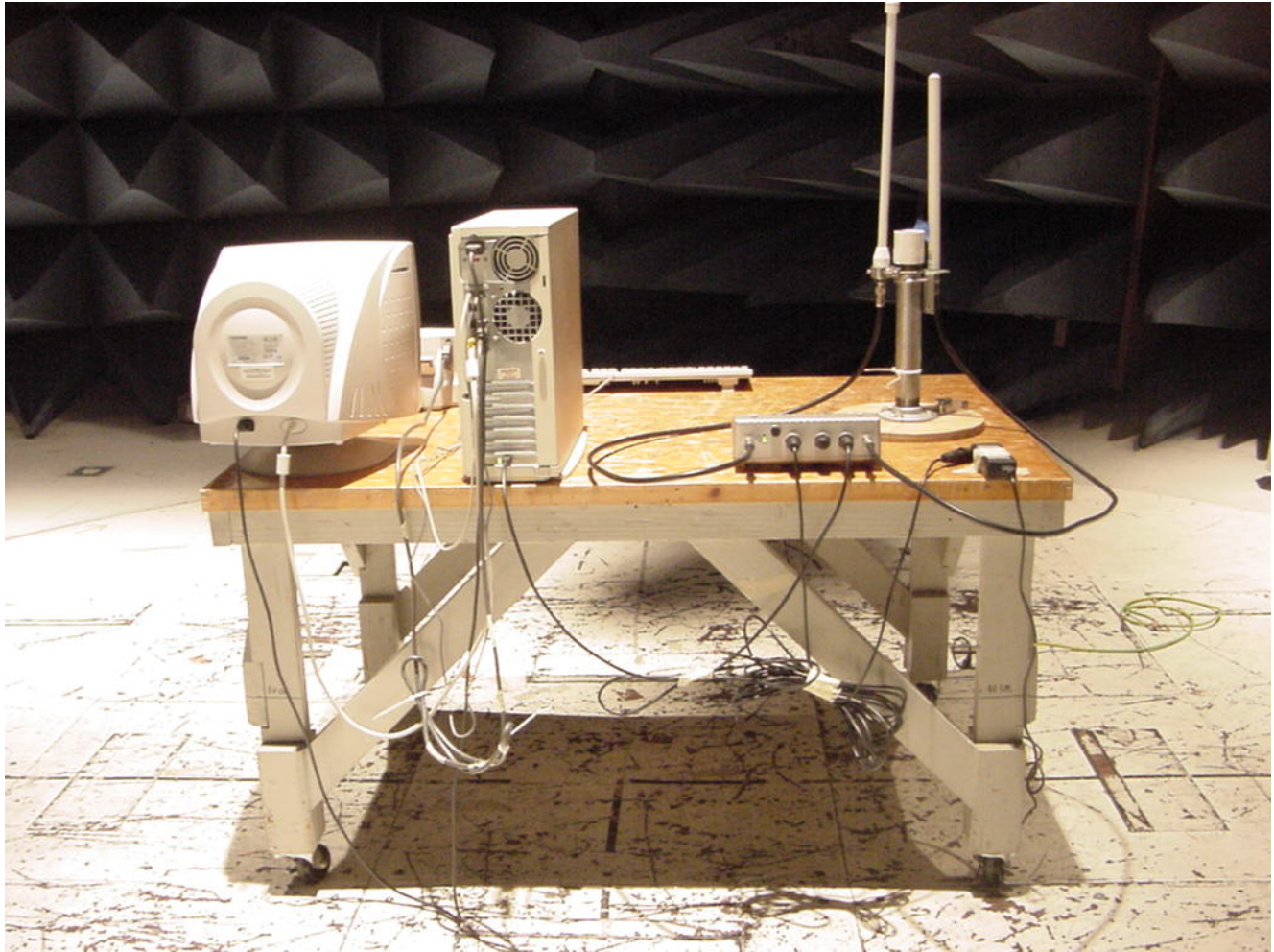
Photograph 2. Radiated Emission Test Setup < 1 GHz
