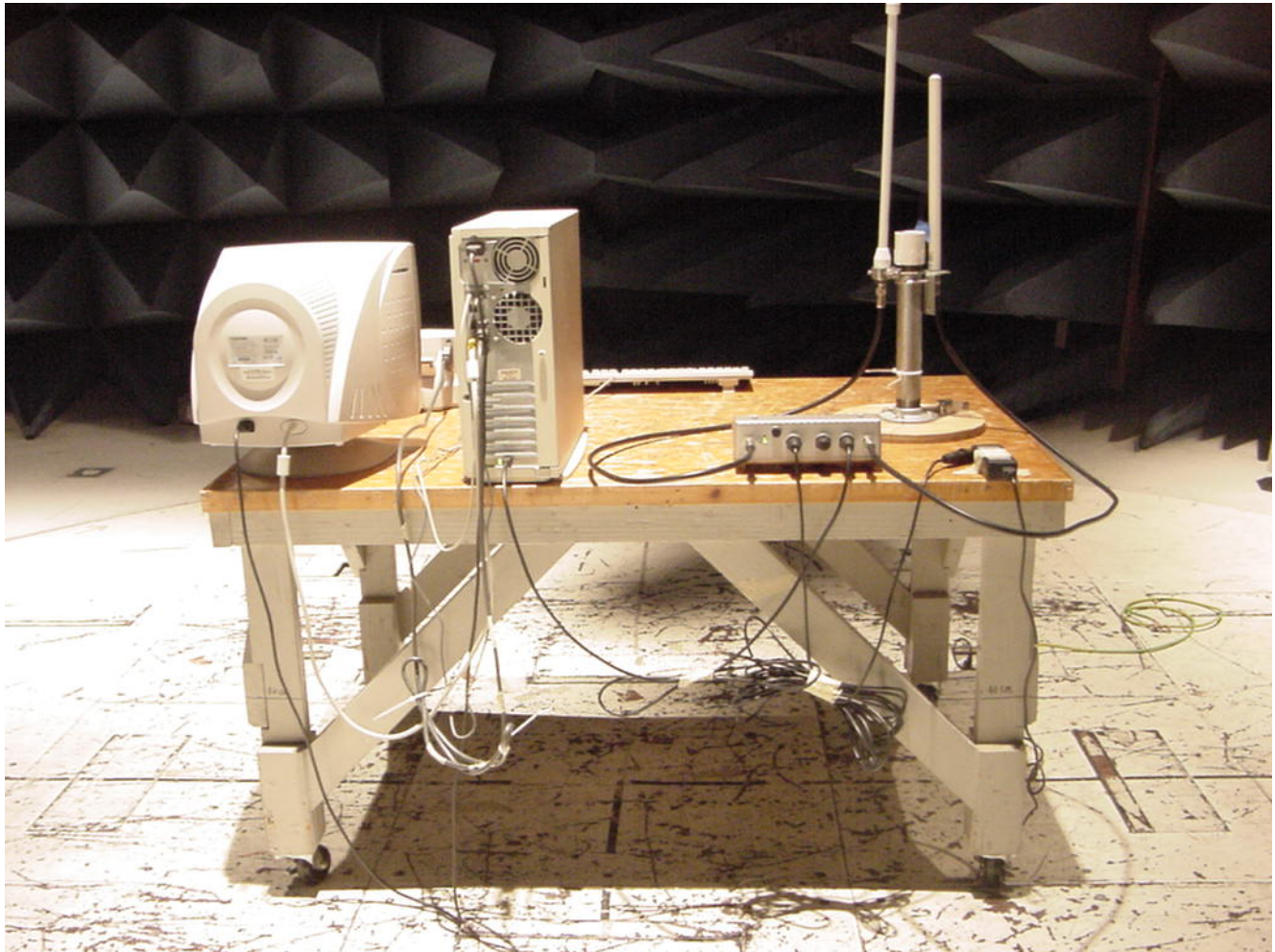
Photograph 2. Radiated Emission Test Setup
