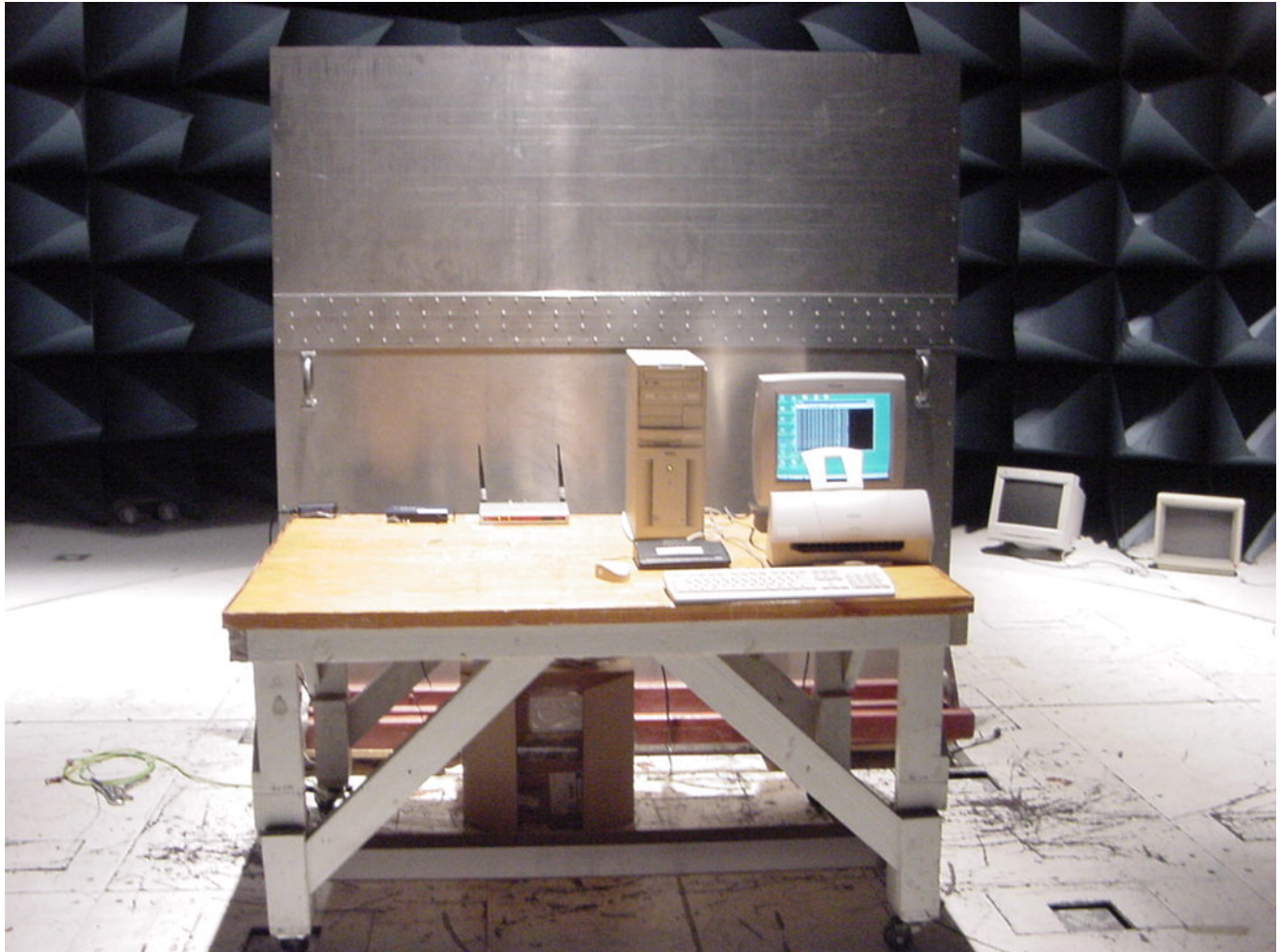
Photograph 1. Conducted Emissions Test Setup
