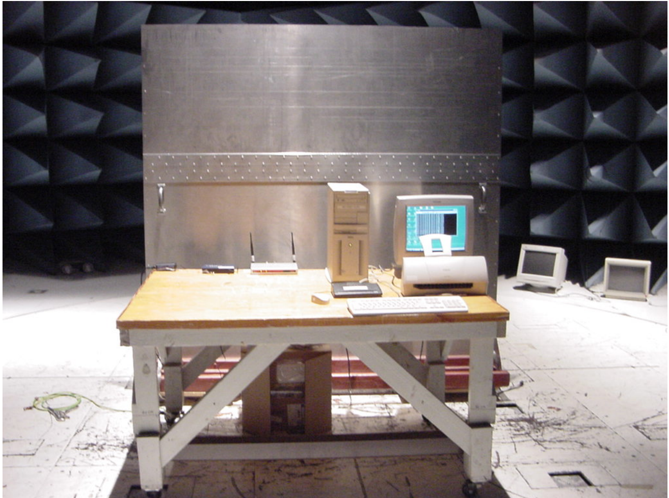
Photograph 1. Conducted Emissions Test Setup
