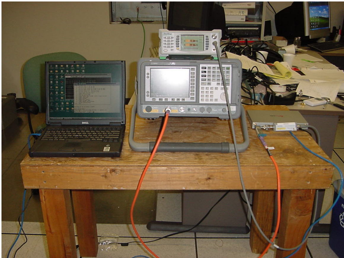
Photograph 3. Spurious Emissions at Antenna Terminals Test Setup
