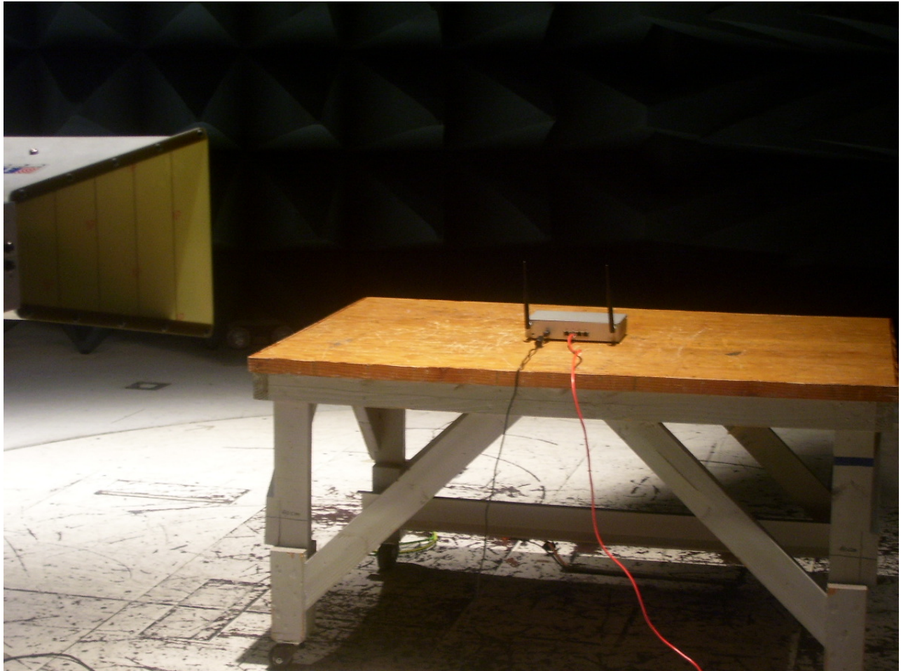
Test Equipment and setup for various Radiated Measurements – Dipole Antenna
