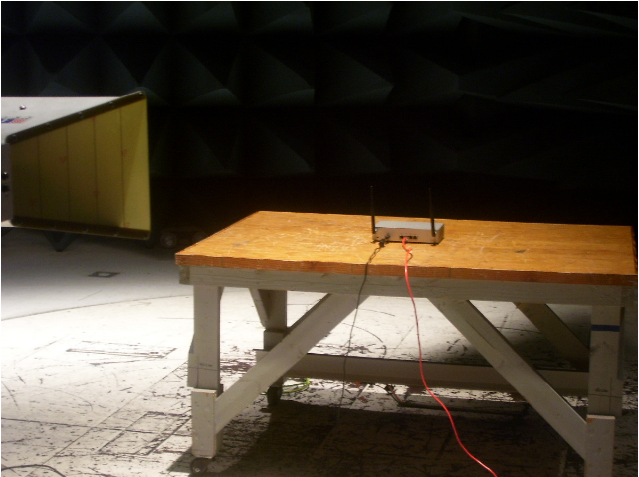
Photograph 4. Test Equipment and setup for various Radiated Measurements – Dipole Antenna
