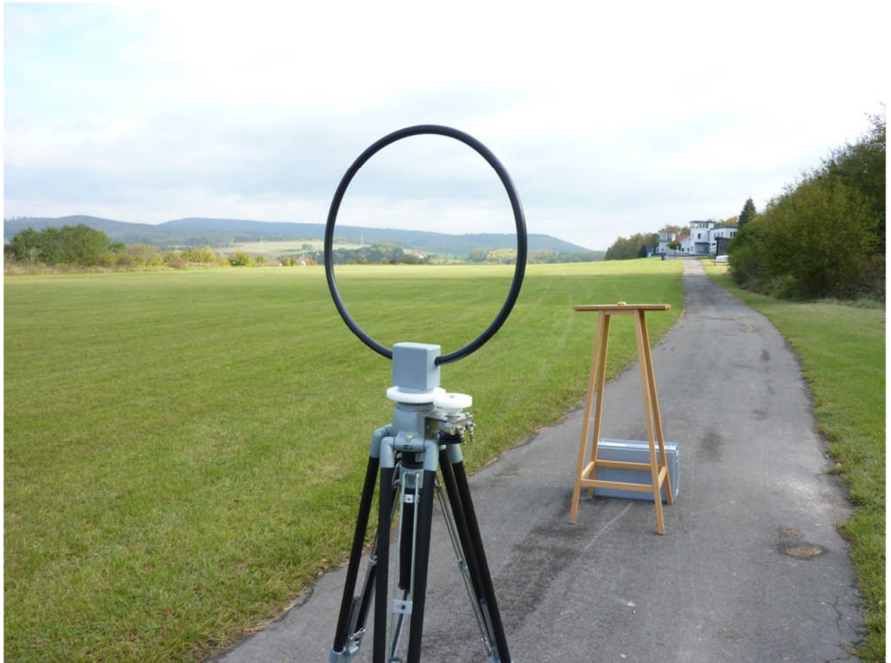
113539emi3.JPG: Test set-up final radiated emission (H-Field)
