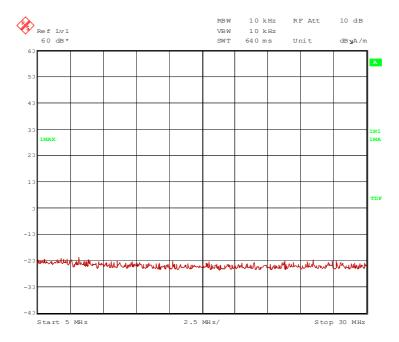
Only the wanted frequency 457 kHz was detected during the measurement. No other significant spurious frequencies above the noise floor of the system were found during the preliminary radiated emission test, so only the wanted frequency-measurement was carried out on the outdoor test site.
