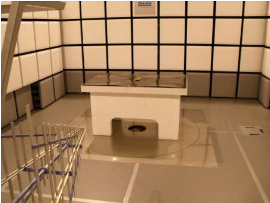
Figure 4: Radiated emission test, 200 MHz – 1 GHz - SAC
