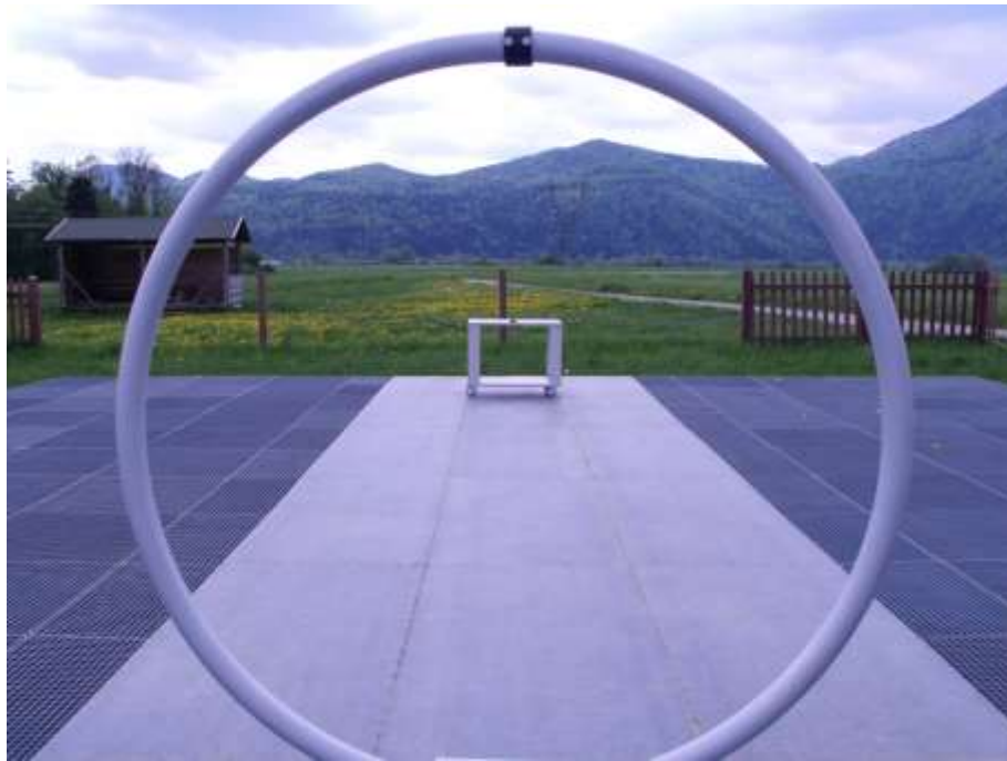
Figure 5: Radiated emission test, 9 kHz – 30 MHz– OATS
