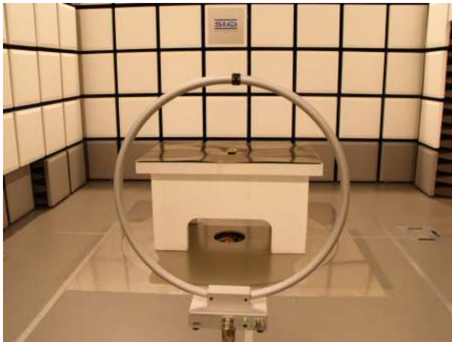
Figure 1: Radiated emission test, 9 kHz – 30 MHz - SAC
