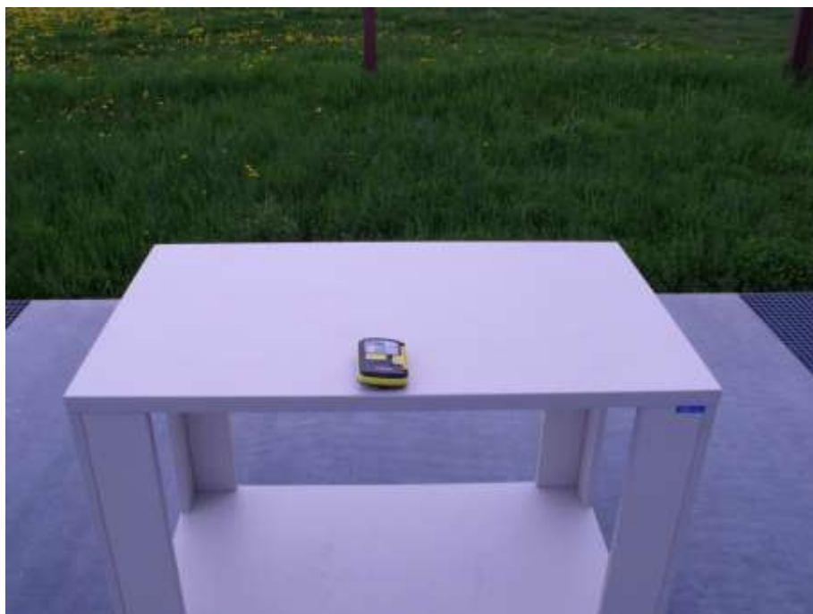
Figure 6: Radiated emission test, 9 kHz – 30 MHz – OATS
