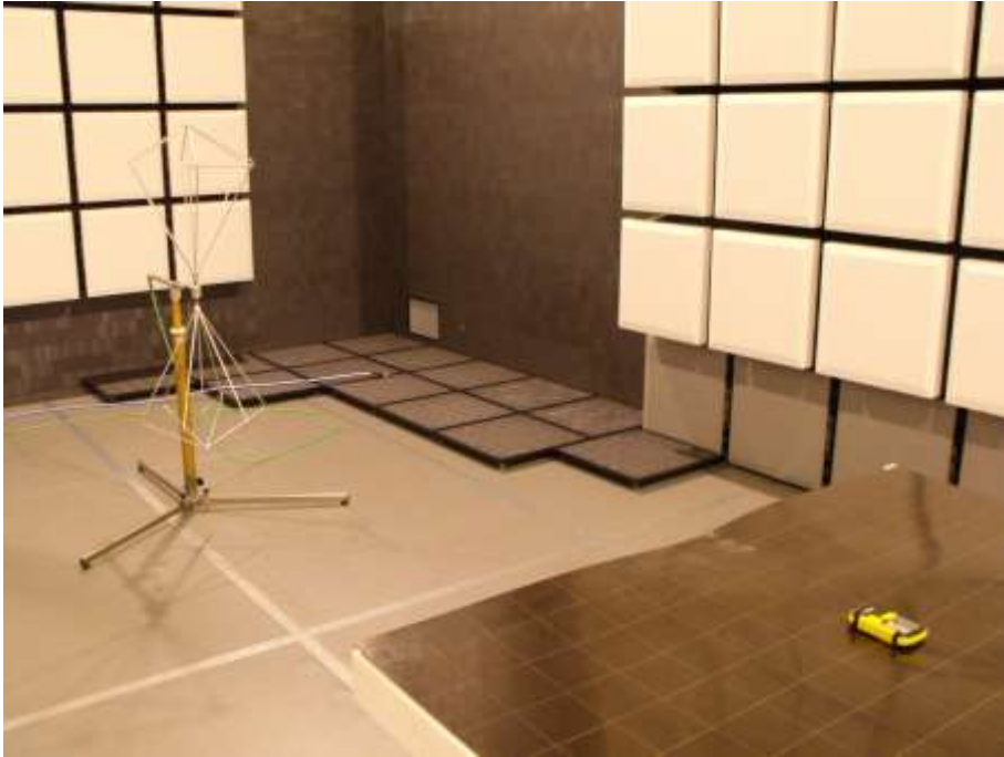
Figure 3: Radiated emission test, 30 MHz – 200 MHz - SAC
