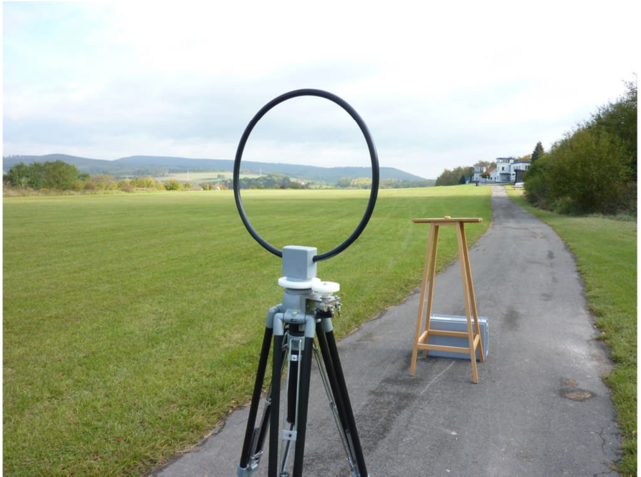
113943emi3.JPG: Test set-up final radiated emission (H-Field)
