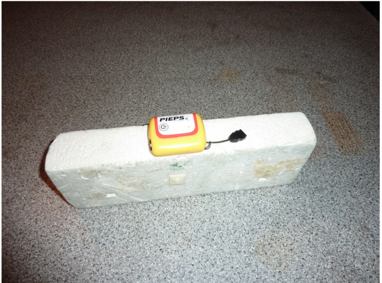
113943emi2.JPG: Test set-up radiated emission (E-Field)
