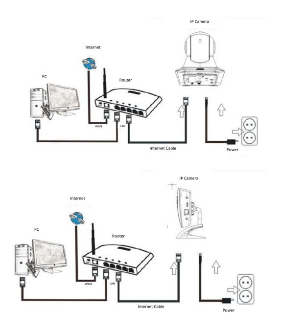
Connect the camera with Internet cable to the router, and with the power cord to the mains, like shown above.
