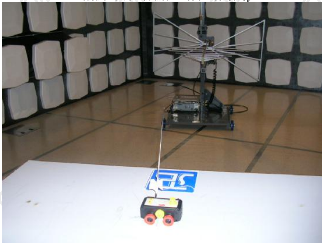
Measurement of Radiated Emission Test Set Up
