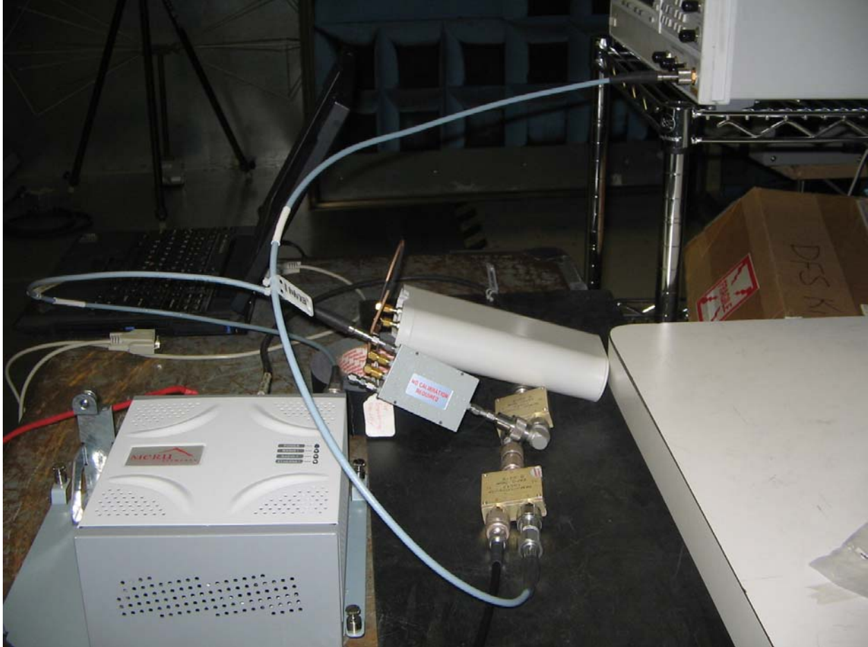
Figure 15, DFS Master test setup
