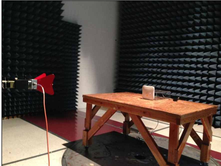
Photograph 10. Radiated Spurious Emissions, Test Setup, Above 1 GHz, Internal Antenna
