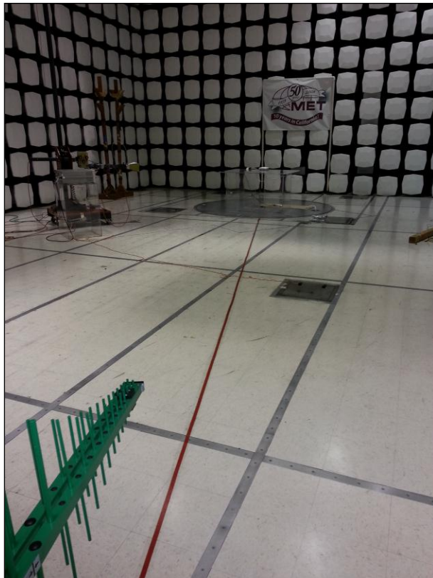
Photograph 4. Radiated Emission, Test Setup, PoE
