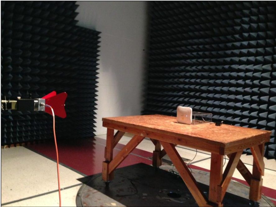
Photograph 10. Radiated Spurious Emissions, Test Setup, Above 1 GHz
