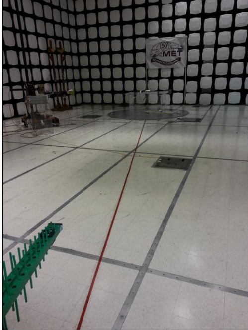
Photograph 3. Radiated Emission, Test Setup, AC-DC Power Supply
