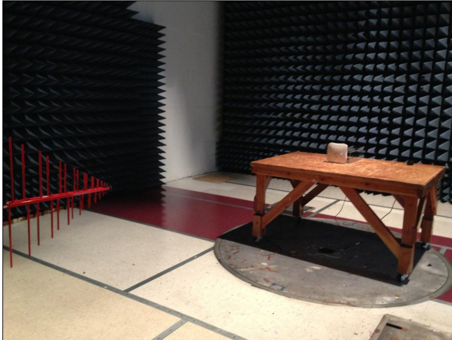
Photograph 9. Radiated Spurious Emissions, Test Setup, 30 MHz – 1 GHz
