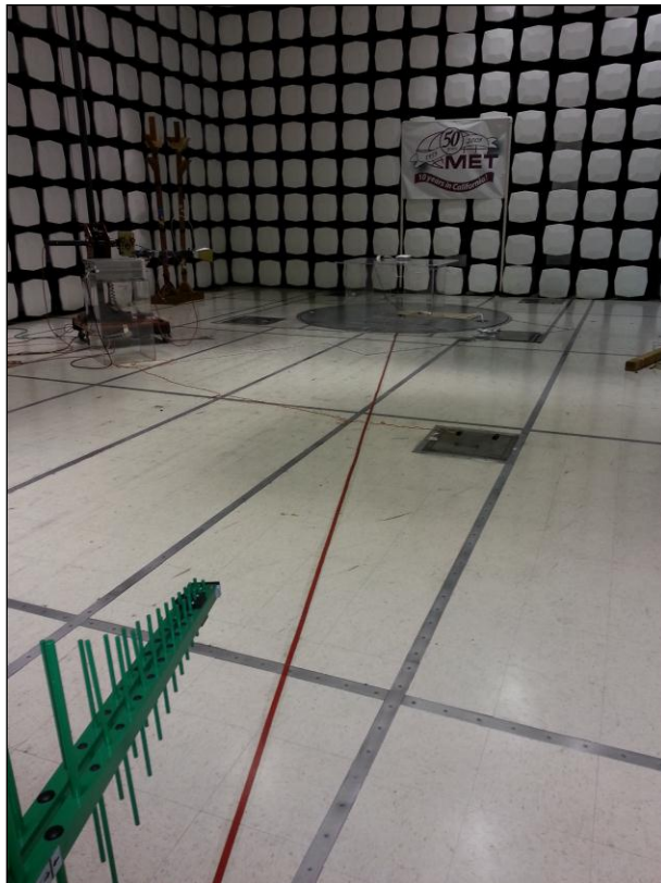
Photograph 4. Radiated Emission, Test Setup, PoE
