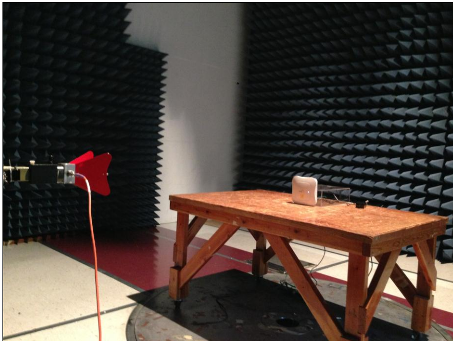
Photograph 10. Radiated Spurious Emissions, Test Setup, Above 1 GHz
