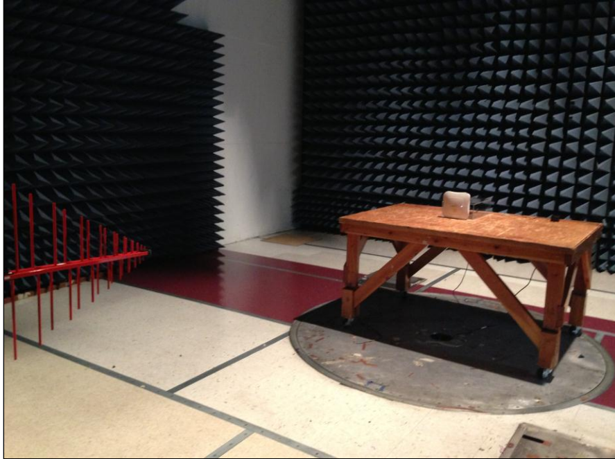
Photograph 7. Radiated Spurious Emissions, Test Setup, 30 MHz – 1 GHz
