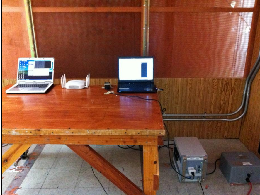
Photograph 3. Conducted Emissions, Test Setup, PoE, 1
