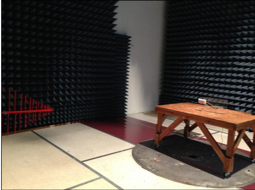
Photograph 9. Radiated Spurious Emissions, Test Setup, 30 MHz – 1 GHz, Ceiling Antenna
