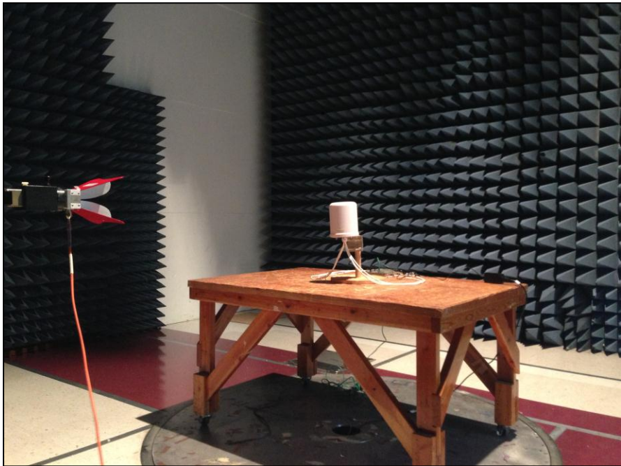
Photograph 12. Radiated Spurious Emissions, Test Setup, Above 1 GHz, Omni Antenna
