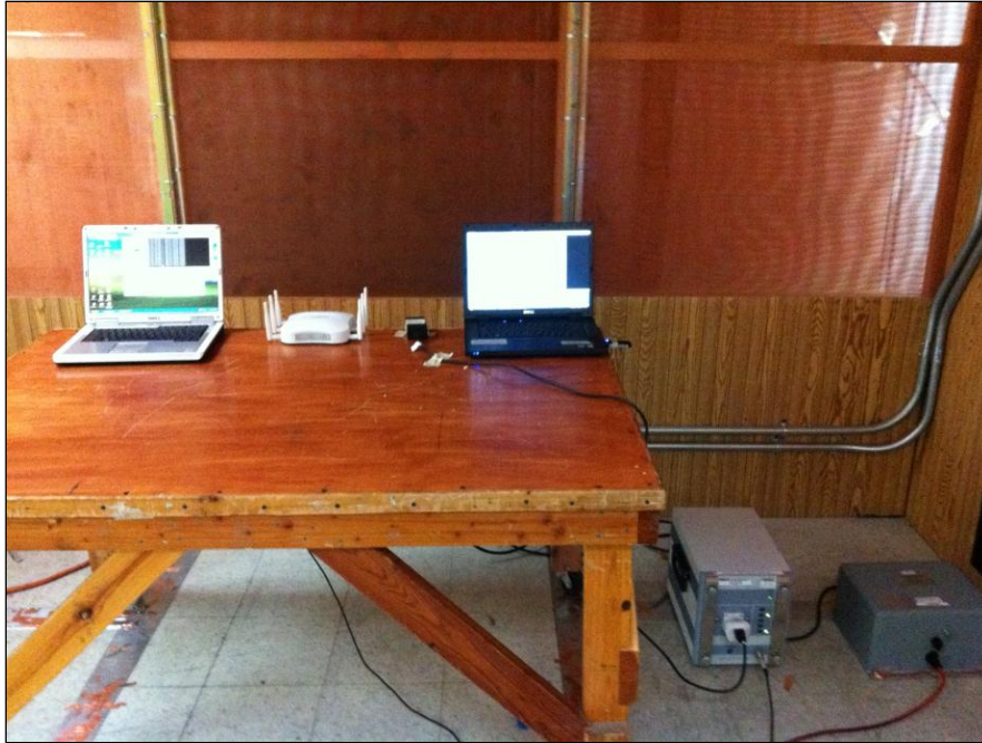
Photograph 1. Conducted Emissions, Test Setup, AC-DC Power Supply, 1
