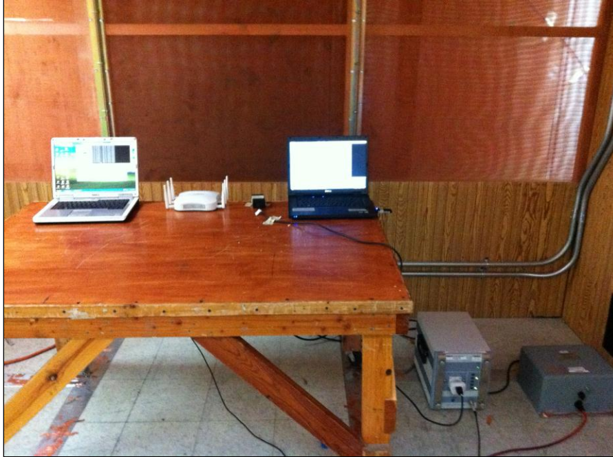
Photograph 7. Conducted Emissions, 15.207(a), Test Setup, AC-DC Power Supply
