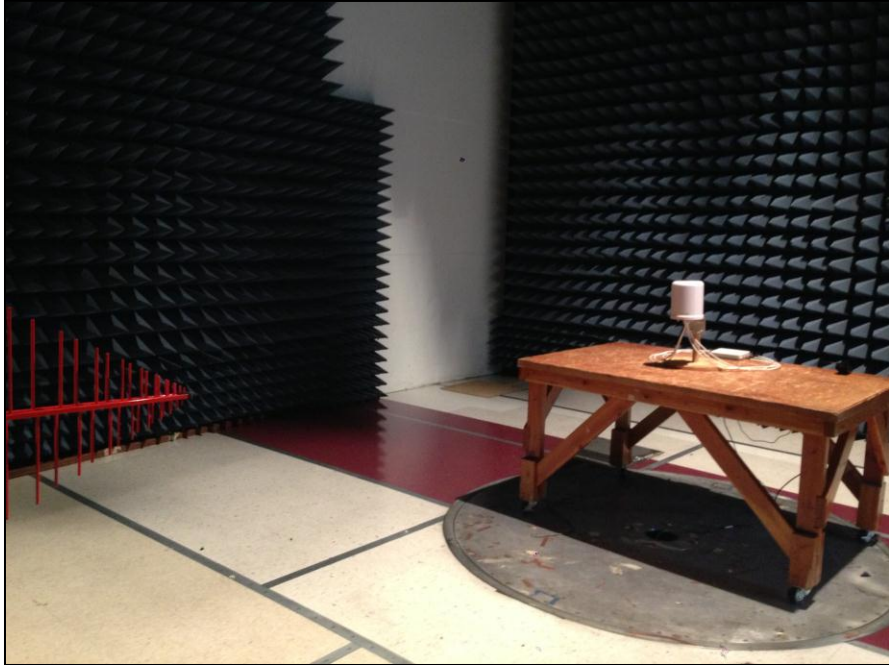
Photograph 11. Radiated Spurious Emissions, Test Setup, 30 MHz – 1 GHz, Omni Antenna
