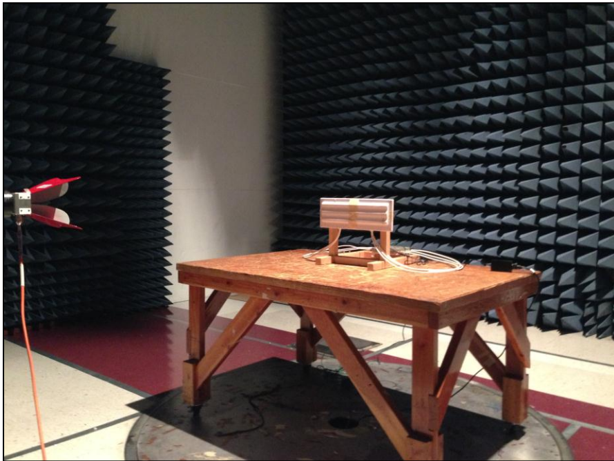
Photograph 14. Radiated Spurious Emissions, Test Setup, Above 1 GHz, Patch Antenna
