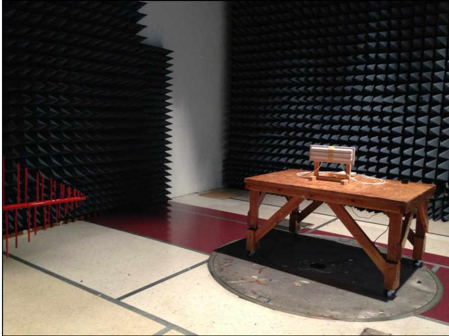
Photograph 13. Radiated Spurious Emissions, Test Setup, 30 MHz – 1 GHz, Patch Antenna
