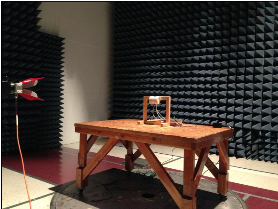
Photograph 10. Radiated Spurious Emissions, Test Setup, Above 1 GHz, Ceiling Antenna
