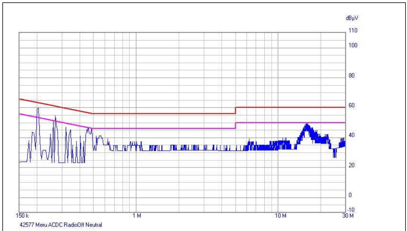
Plot 12. Conducted Emissions, 15.207(a), Neutral Line, AC/DC
