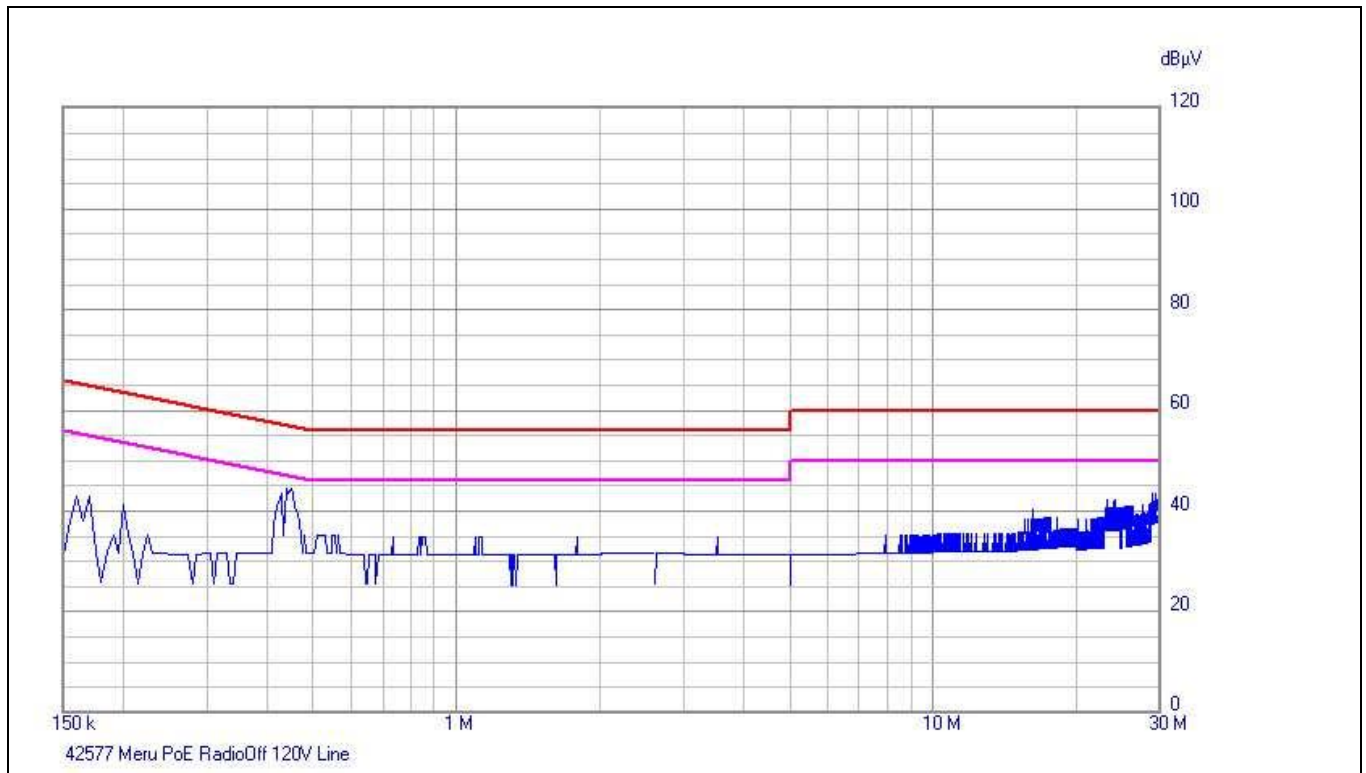
Plot 9. Conducted Emissions, 15.207(a), Phase Line, PoE
