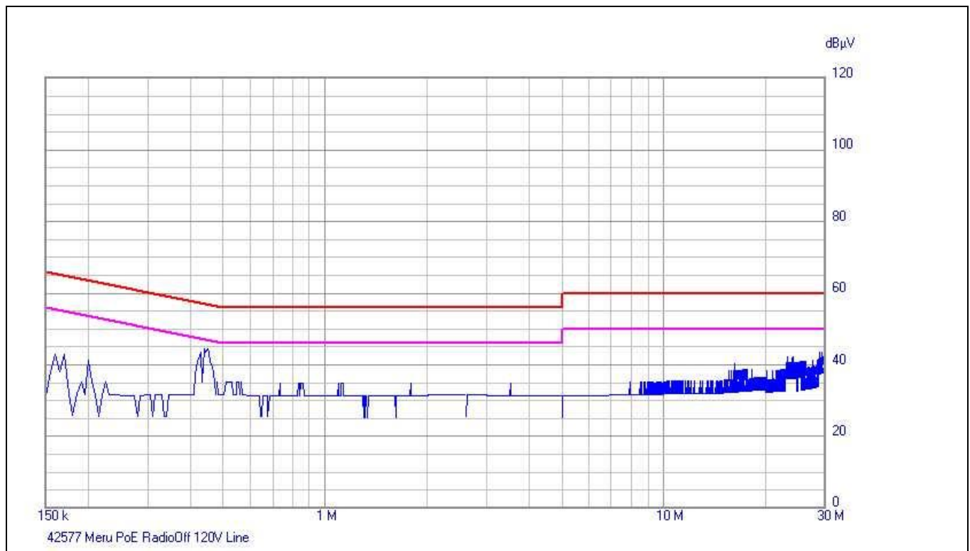
Plot 1. Conducted Emissions, Phase Line, PoE
