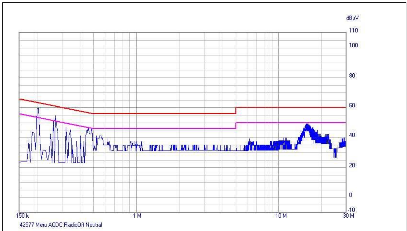
Plot 4. Conducted Emissions, Neutral Line, AC/DC
