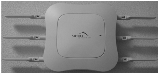
Figure 14: Horizontal Antenna Orientation (Side View)
