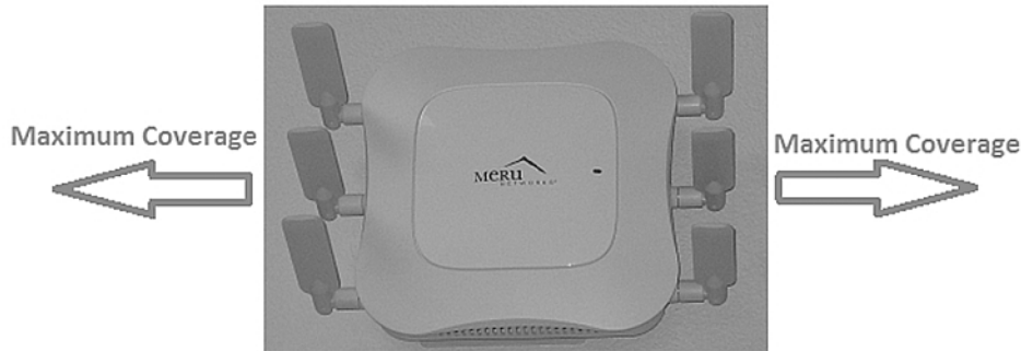
Figure 12: Vertical Antenna Orientation
