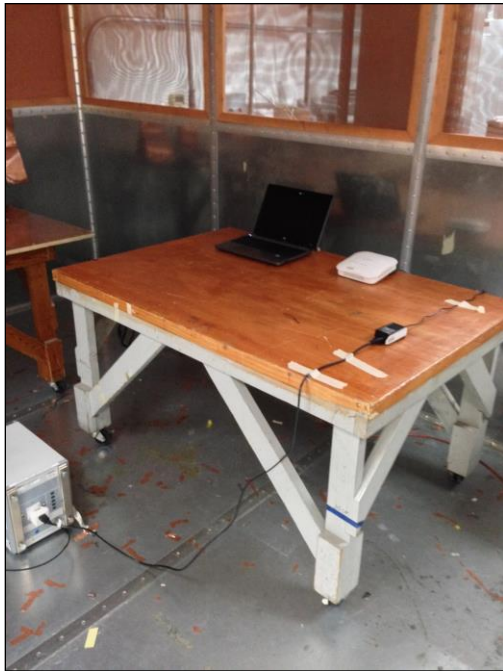
Photograph 2. Conducted Emissions, Test Setup, AC/DC
