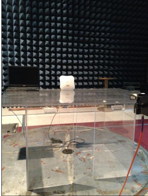
Photograph 7. Radiated Spurious Emissions, Test Setup, 18-40 GHz
