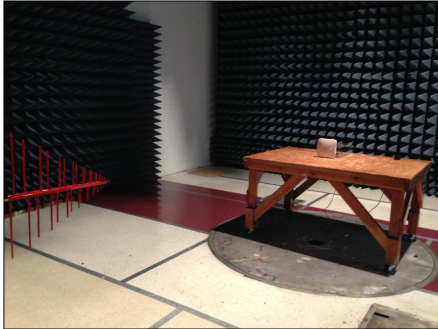
Photograph 9. Radiated Spurious Emissions, Test Setup, 30 MHz – 1 GHz, Internal Antenna
