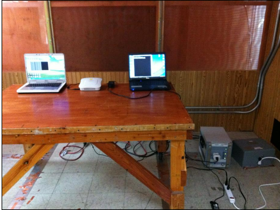
Photograph 2. Conducted Emissions, Test Setup, AC-DC Power Supply
