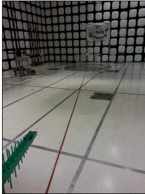
Photograph 4. Radiated Emission, Test Setup, AC-DC Power Supply
