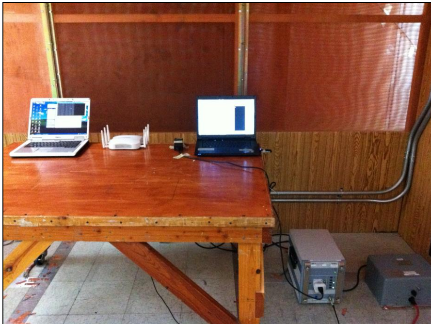
Photograph 8. Conducted Emissions, 15.207(a), Test Setup, PoE
