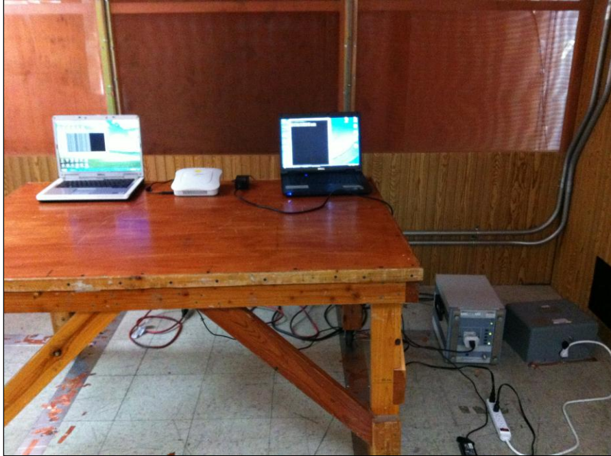
Photograph 5. Conducted Emissions, 15.207(a), Test Setup, AC-DC Power Supply
