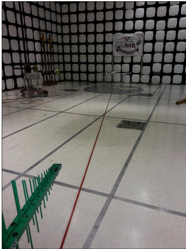
Photograph 4. Radiated Emission, Test Setup, PoE
