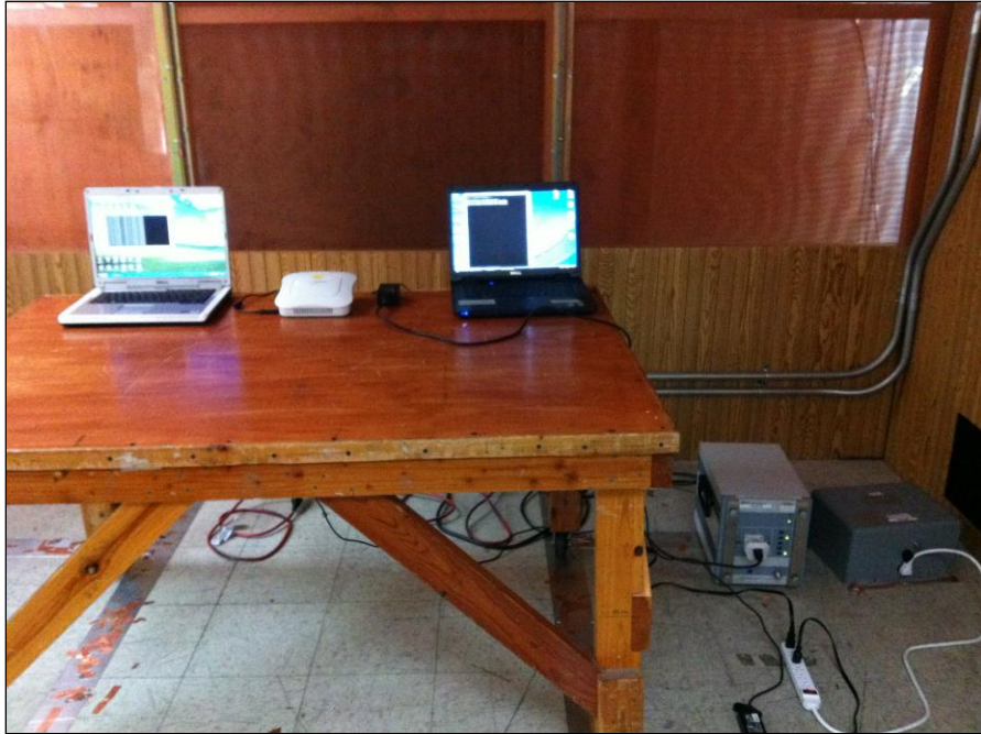
Photograph 1. Conducted Emissions, Test Setup, AC-DC Power Supply
