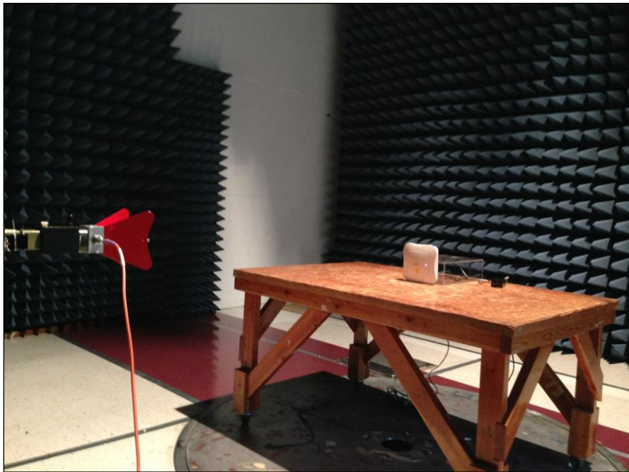
Photograph 8. Radiated Spurious Emissions, Test Setup, Above 1 GHz
