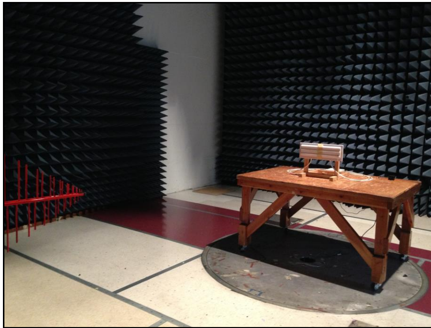
Radiated Spurious Emissions, Patch Antenna, Test Setup, 30 MHz – 1 GHz
