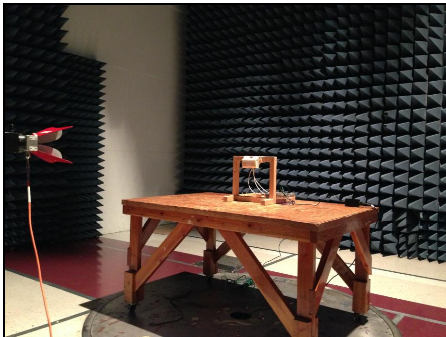
Photograph 7. Radiated Spurious Emissions, Ceiling Antenna, Test Setup, 1 GHz – 18 GHz
