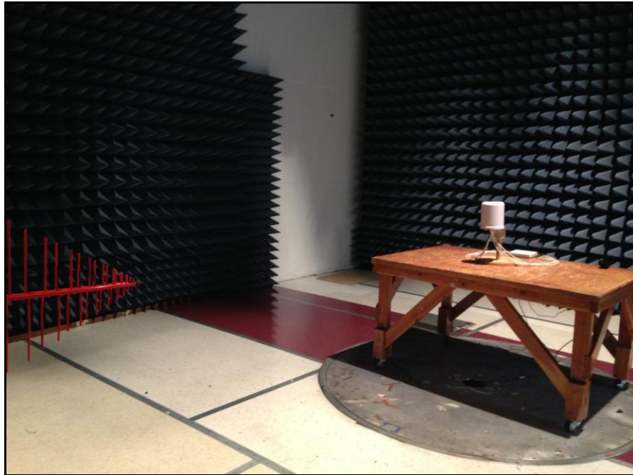
Photograph 8. Radiated Spurious Emissions, Omni Antenna, Test Setup, 30 MHz – 1 GHz
