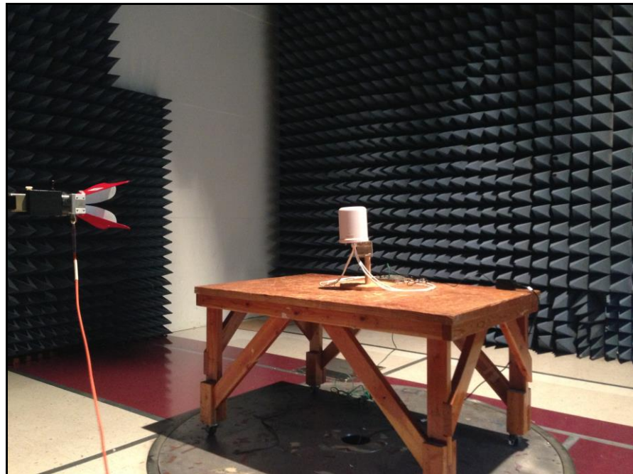
Photograph 9. Radiated Spurious Emissions, Omni Antenna, Test Setup, 1 GHz – 18 GHz
