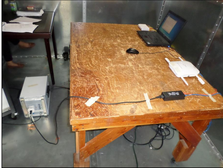
Photograph 2. Conducted Emissions, Test Setup, PoE
