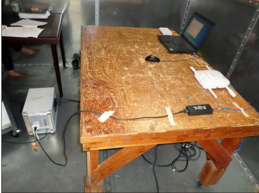
Photograph 1. Conducted Emissions, Test Setup, PoE
