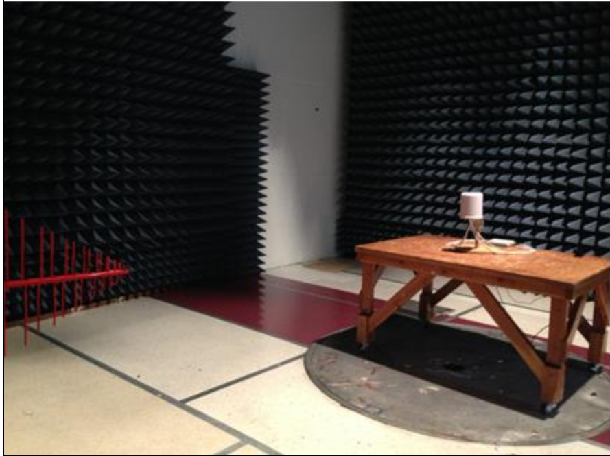
Photograph 7. Radiated Spurious Emissions, Test Setup, 30 MHz – 1 GHz, Omni Antenna
