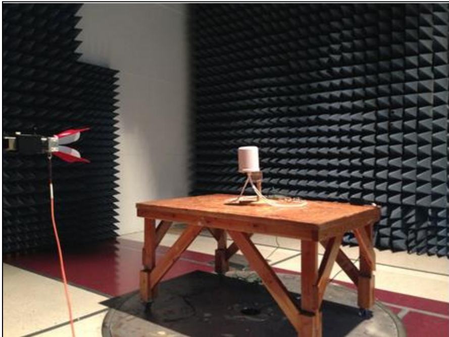
Photograph 8. Radiated Spurious Emissions, Test Setup, Above 1 GHz, Omni Antenna
