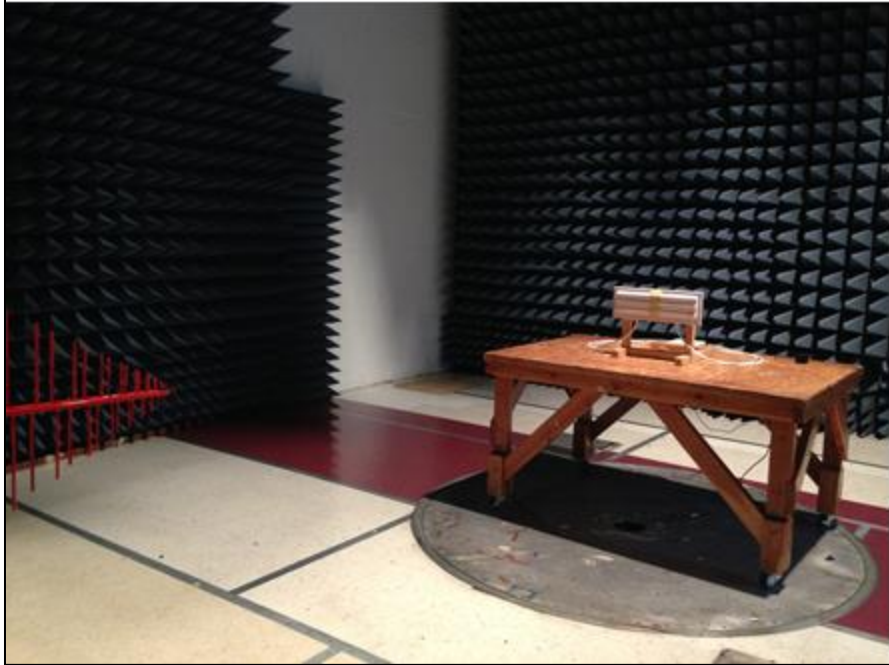
Photograph 9. Radiated Spurious Emissions, Test Setup, 30 MHz – 1 GHz, Patch Antenna
