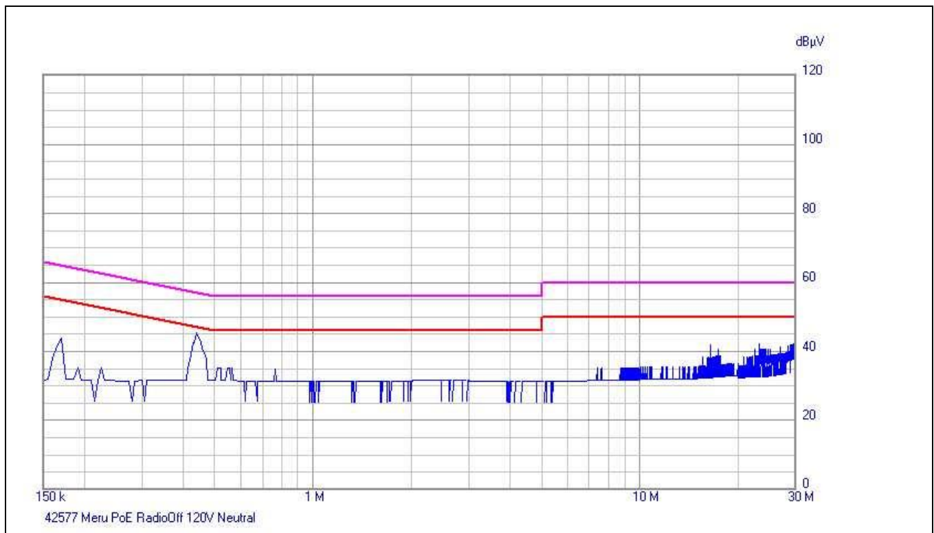
Plot 10. Conducted Emissions, 15.207(a), Neutral Line, PoE
