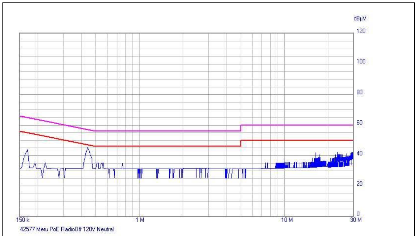
Plot 2. Conducted Emissions, Neutral Line, PoE
