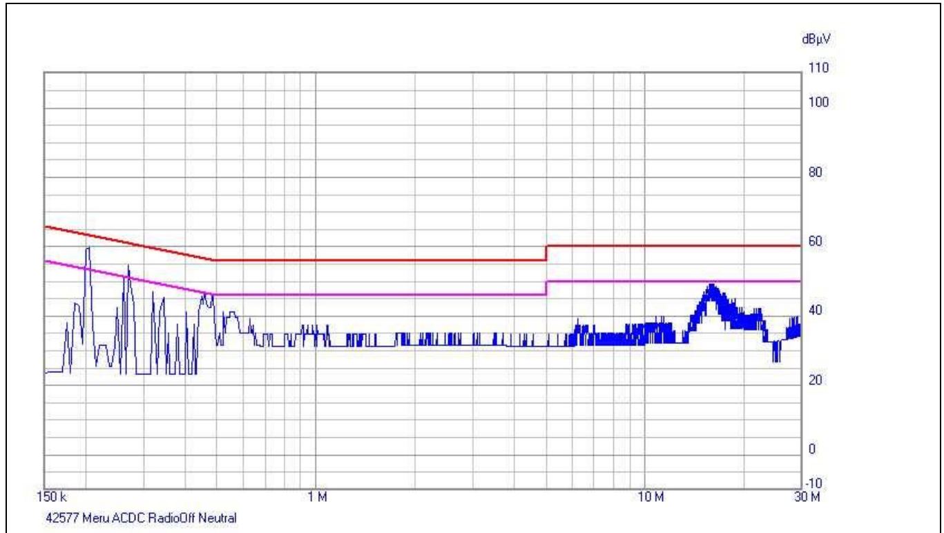
Plot 4. Conducted Emissions, Neutral Line, AC/DC
