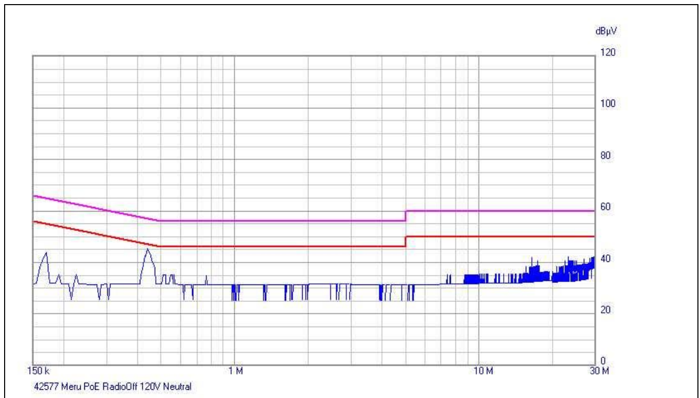
Plot 10. Conducted Emissions, 15.207(a), Neutral Line, PoE
