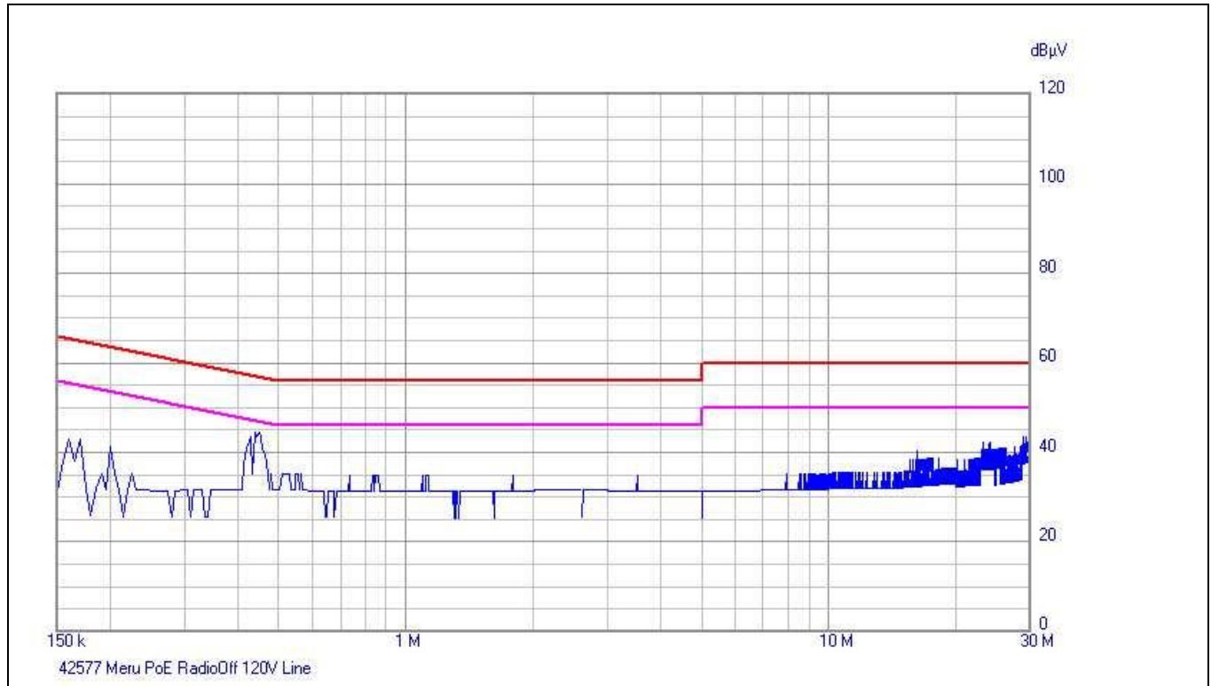
Plot 1. Conducted Emissions, Phase Line, PoE
