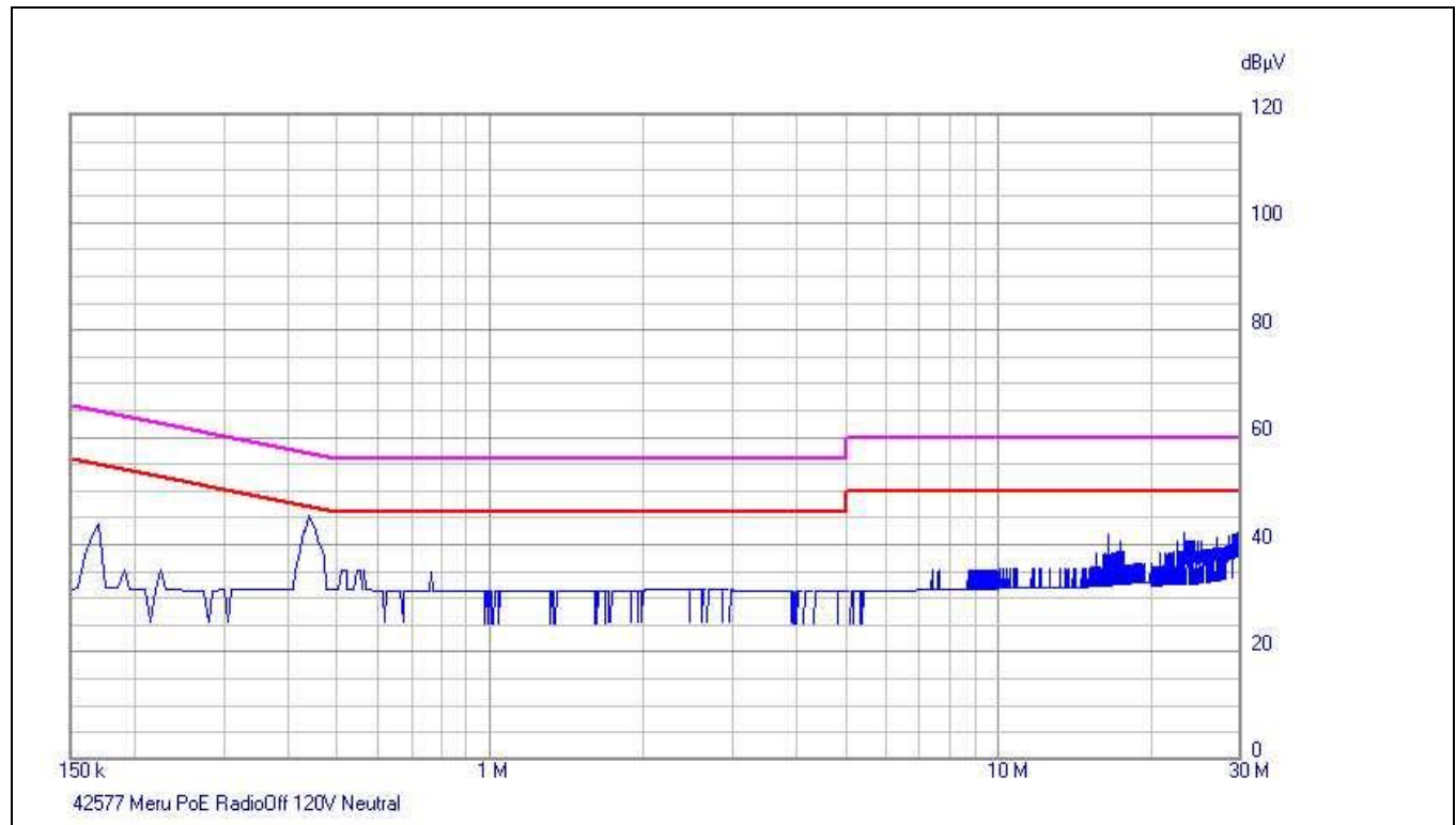
Plot 10. Conducted Emissions, 15.207(a), Neutral Line, PoE
