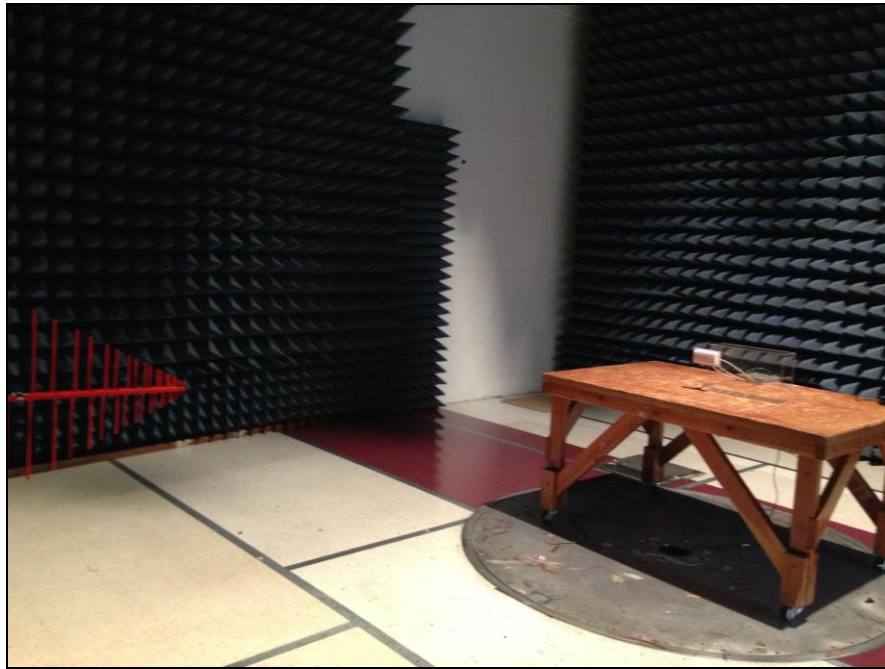
Photograph 11. Radiated Spurious Emissions, Test Setup, 30 MHz – 1 GHz, Ceiling Antenna
