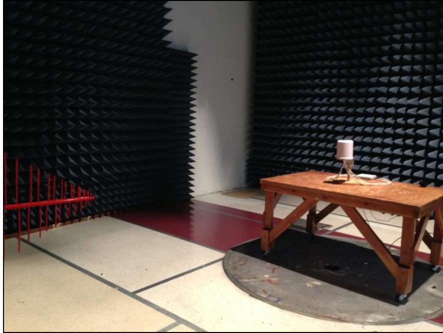
Photograph 13. Radiated Spurious Emissions, Test Setup, 30 MHz – 1 GHz, Omni
