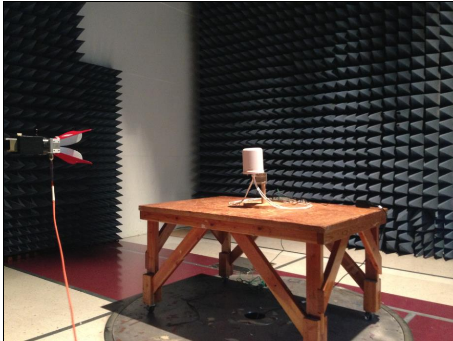
Photograph 14. Radiated Spurious Emissions, Test Setup, Above 1 GHz, Omni
