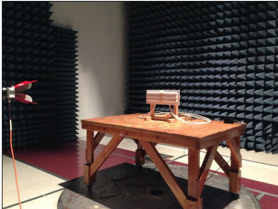
Photograph 16. Radiated Spurious Emissions, Test Setup, Above 1 GHz, Patch Antenna
