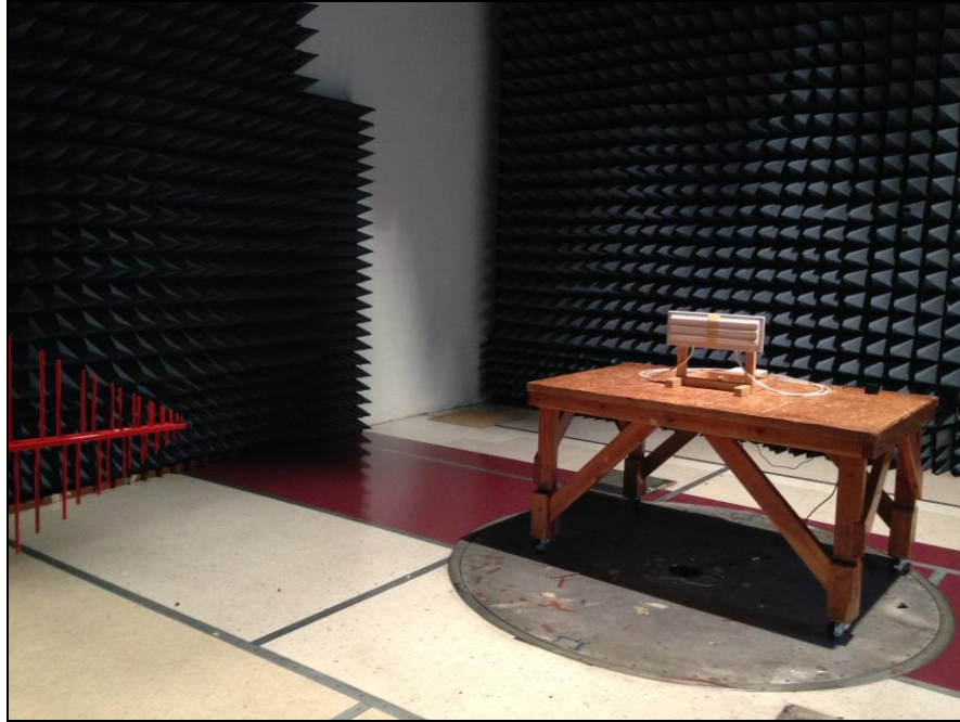
Photograph 15. Radiated Spurious Emissions, Test Setup, 30 MHz – 1 GHz, Patch Antenna
