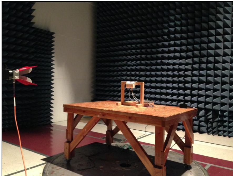
Photograph 12. Radiated Spurious Emissions, Test Setup, Above 1 GHz, Ceiling Antenna
