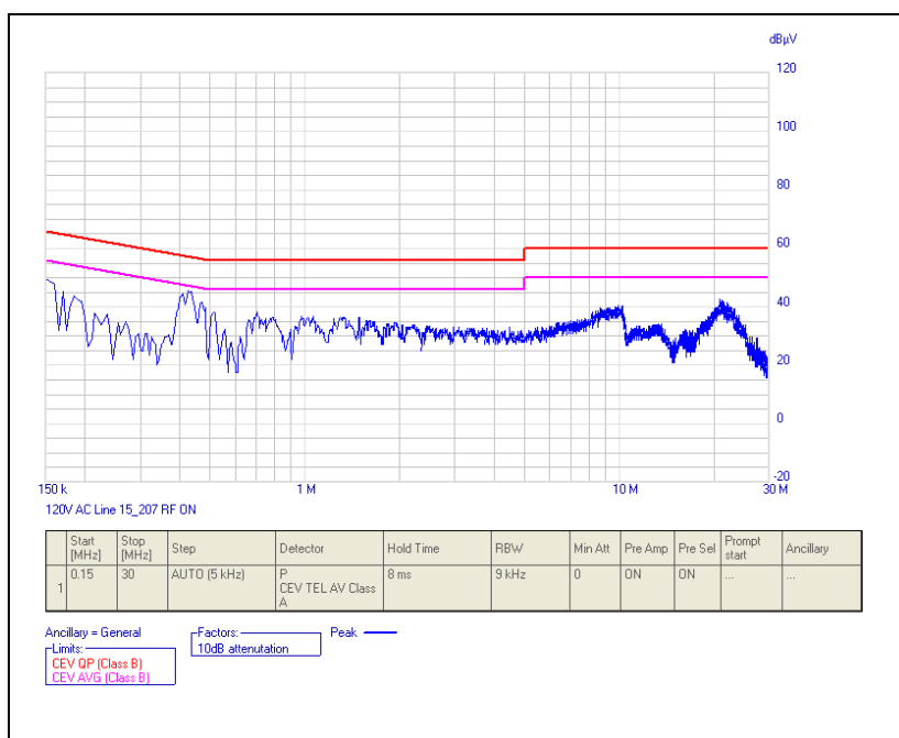
Plot 13. Conducted Emissions, 15.207(a), Phase Line, PoE
