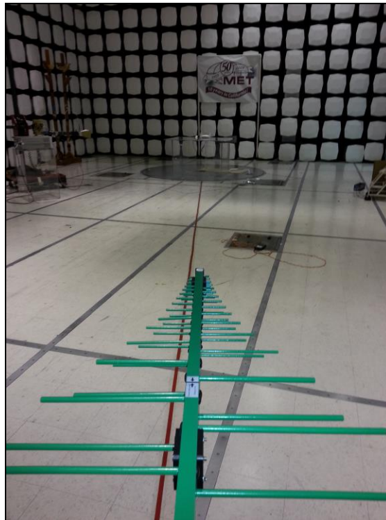
Photograph 6. Radiated Emission, Test Setup, AC-DC Power Supply
