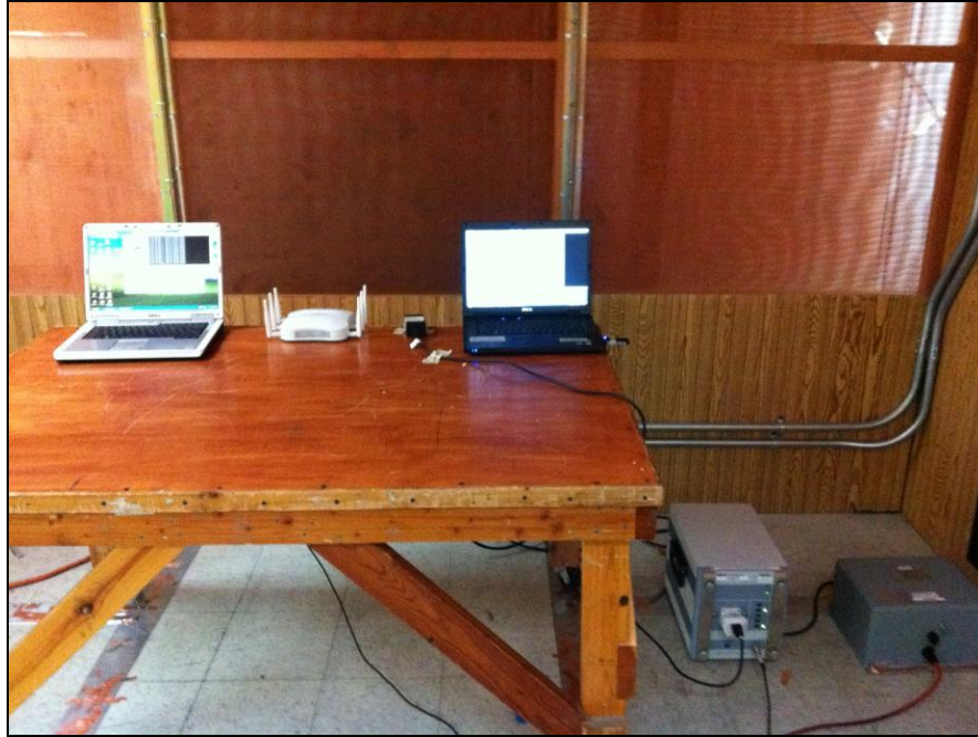
Photograph 2. Conducted Emissions, Test Setup, AC-DC Power Supply, 1
