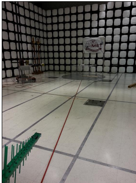
Photograph 7. Radiated Emission, Test Setup, PoE
