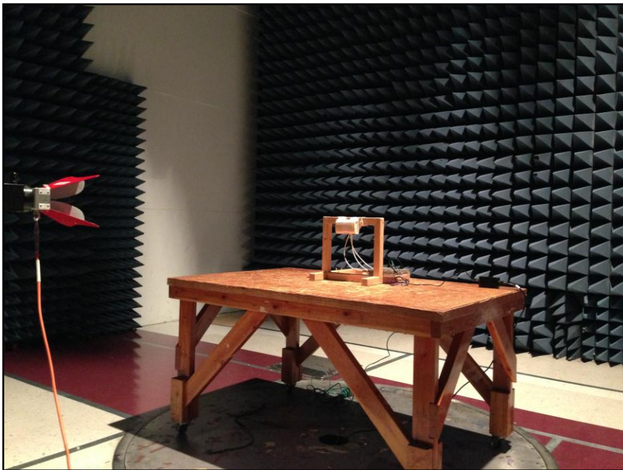
Photograph 10. Radiated Spurious Emissions, Ceiling Antenna, Test Setup, 1 GHz – 18 GHz
