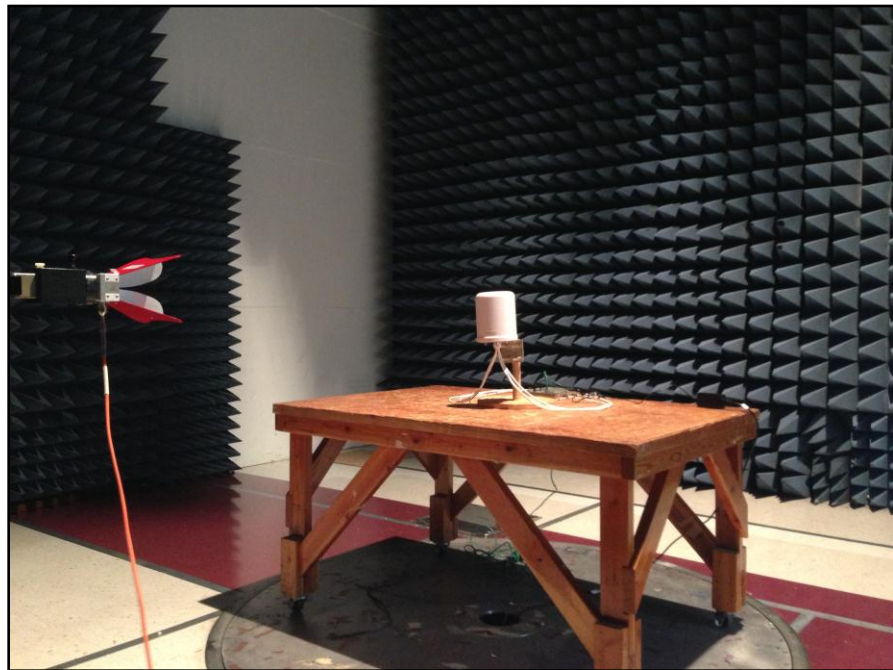
Photograph 12. Radiated Spurious Emissions, Omni Antenna, Test Setup, 1 GHz – 18 GHz
