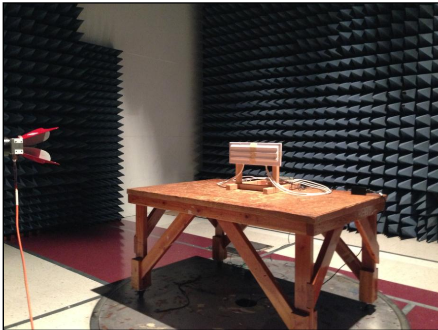
Photograph 14. Radiated Spurious Emissions, Patch Antenna, Test Setup, 1 GHz – 18 GHz
