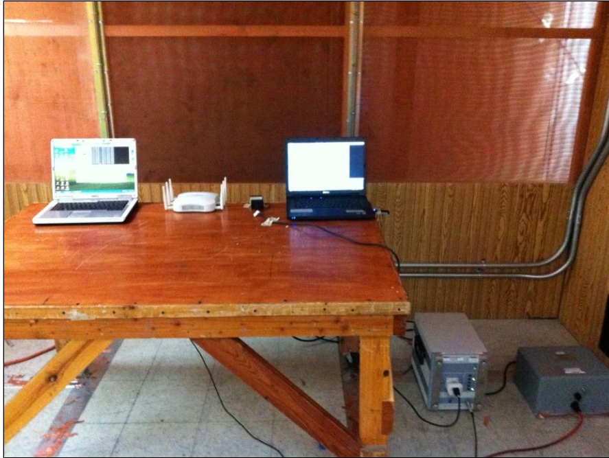
Photograph 1. Conducted Emissions, Test Setup, AC-DC Power Supply, 1
