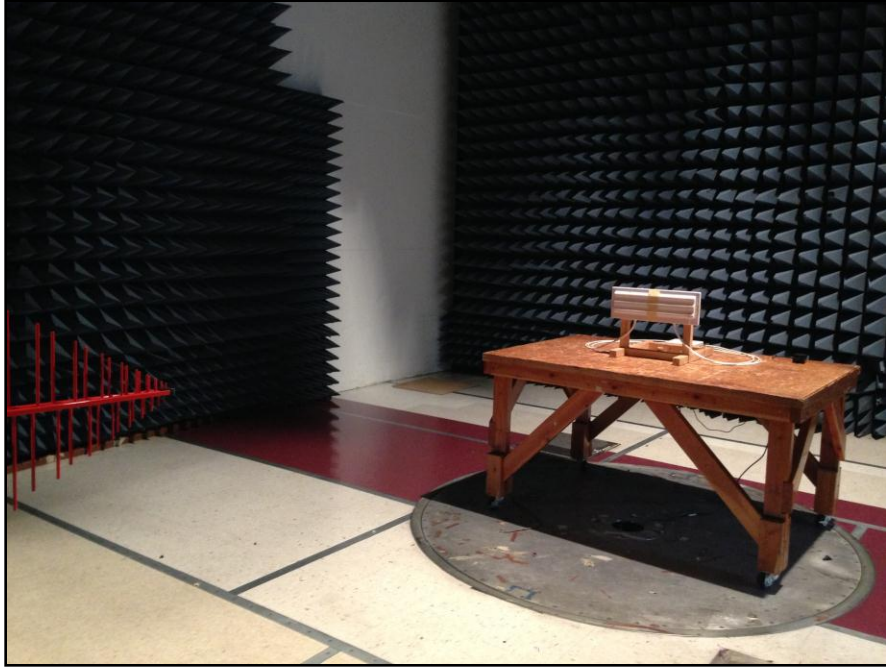
Photograph 13. Radiated Spurious Emissions, Patch Antenna, Test Setup, 30 MHz – 1 GHz
