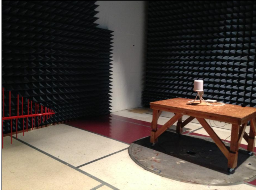
Photograph 11. Radiated Spurious Emissions, Omni Antenna, Test Setup, 30 MHz – 1 GHz
