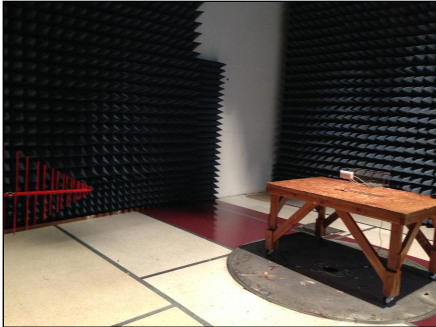
Photograph 9. Radiated Spurious Emissions, Ceiling Antenna, Test Setup, 30 MHz – 1 GHz
