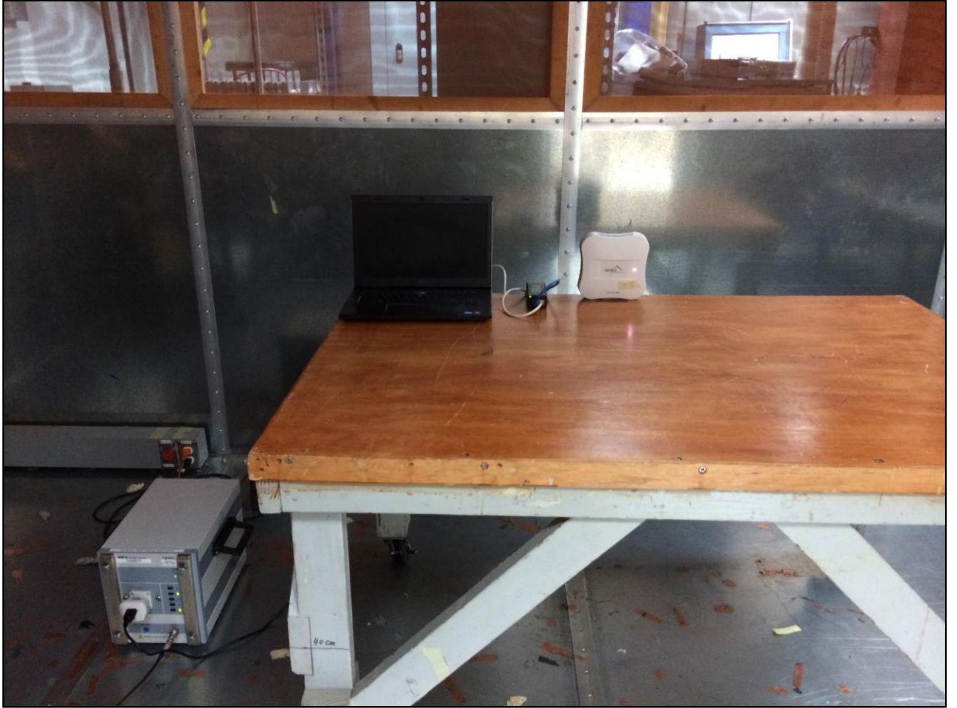
Photograph 1. Conducted Emissions, 15.207(a), Test Setup
