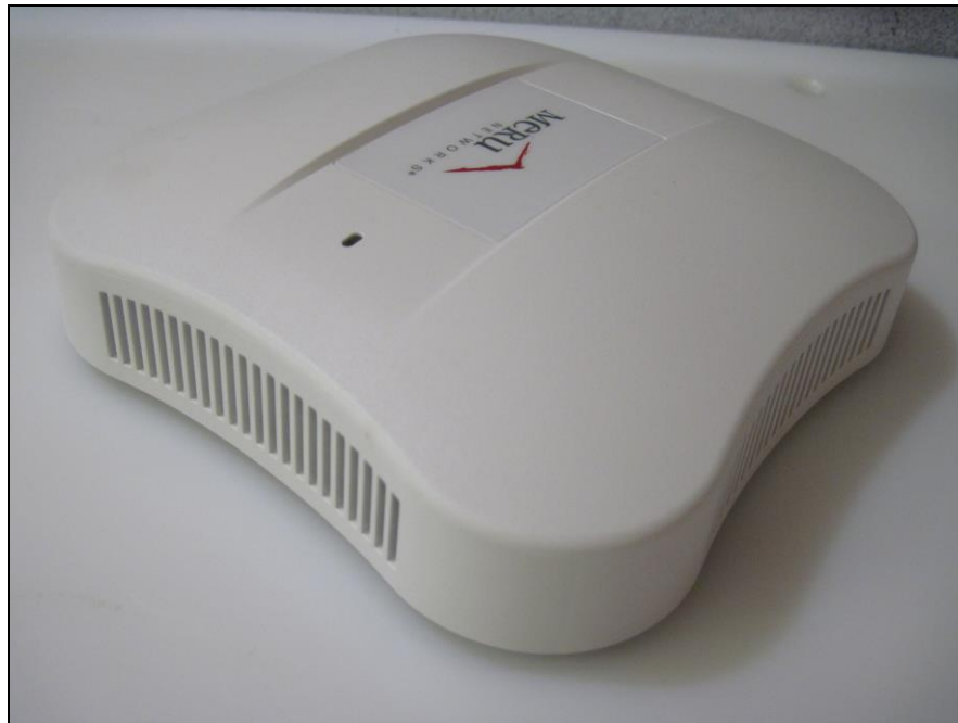
Photograph 1. Meru Networks, Inc. Dual Radio 802.11abgn 3x3 Access Point with internal antenna – AP332i
