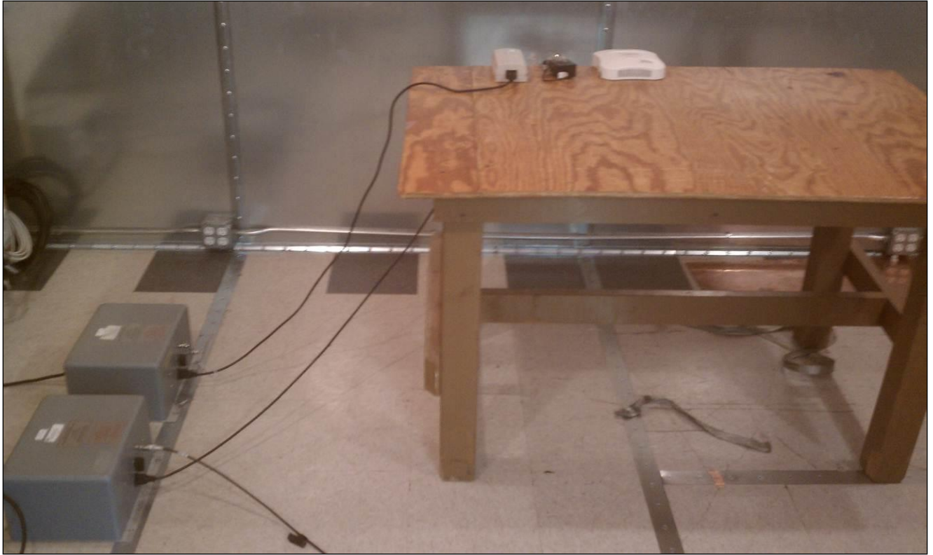
Photograph 1. Conducted Emissions, Test Setup
