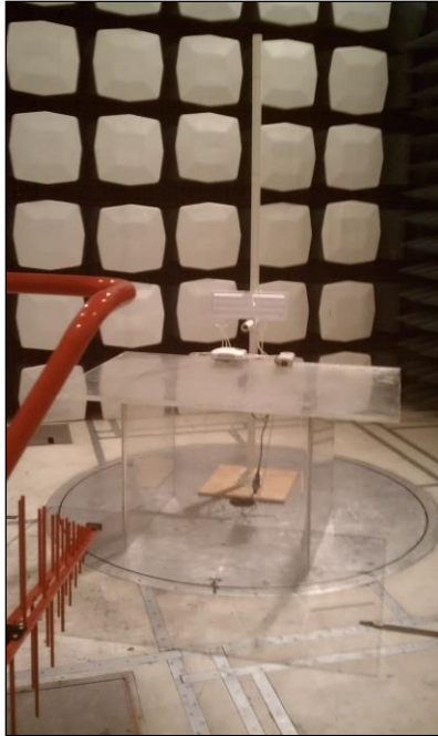
Photograph 7. Radiated Spurious Emissions, Test Setup, LF Patch Antenna
