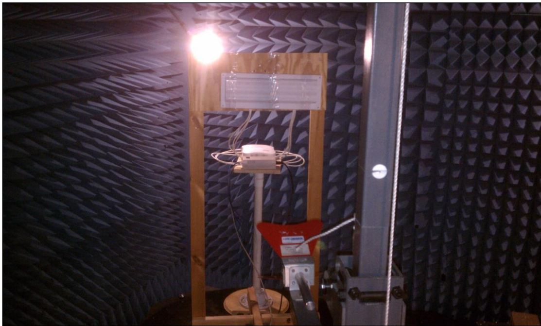
Photograph 8. Radiated Spurious Emissions, Test Setup, HF Patch Antenna
